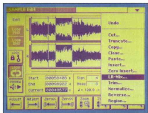
FIG. 3: The stereo waveform editor lacks crossfade looping, but automatic zero-crossing detection and bidirectional loop support help to compensate.
