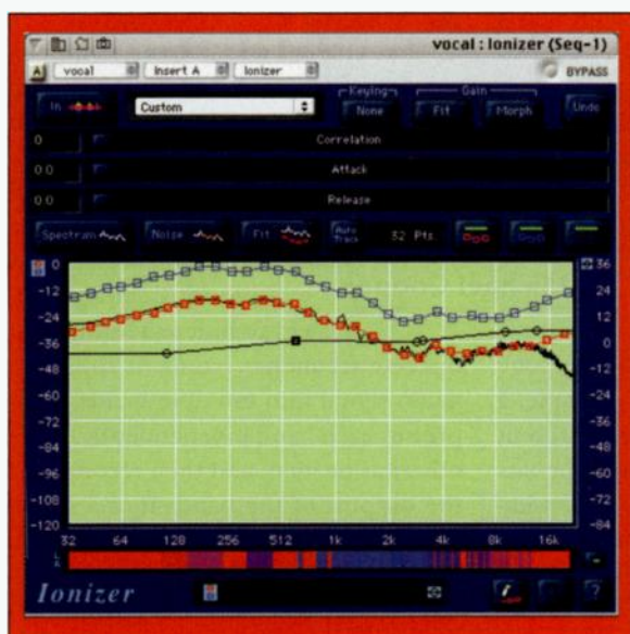
FIG. 1: The Arboretum Systems Ionizer applies dynamics processing across 512 discrete frequency bands.
