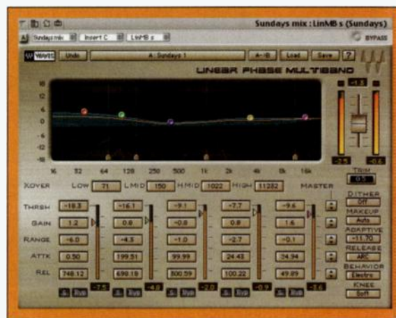
FIG. 8: Waves Linear Phase Multiband offers five independent bands of processing, ultratransparent sound, and a feature-rich interface.
