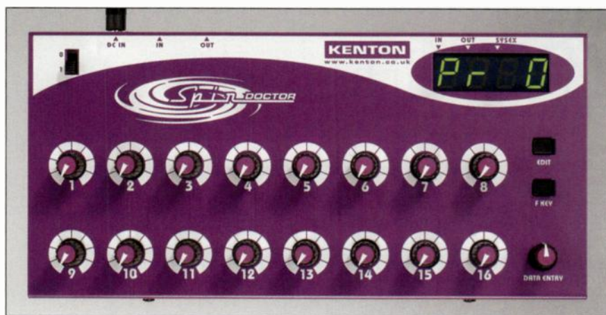
The Kenton Spin Doctor is a MIDI control surface with 16 programmable knobs.
