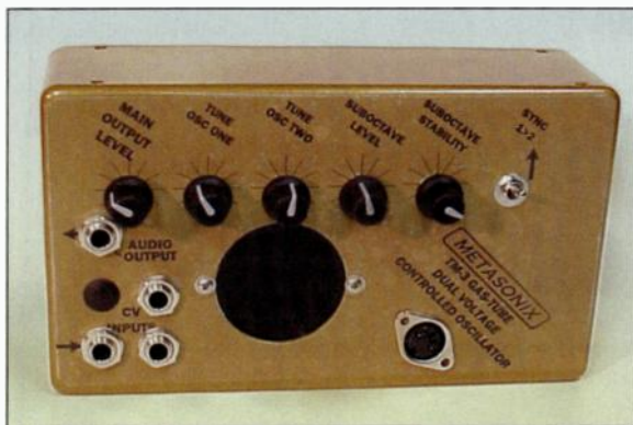
The Metasonix TM-3 is a tube-based dual VCO with a rich sound that can be used to create unique synth textures.
