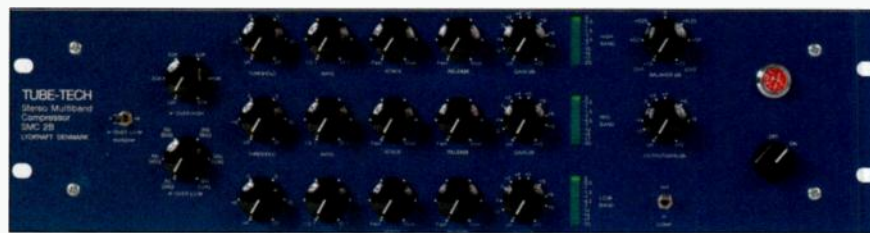
FIG. 6: The 3-band Tube-Tech SMC 2B is the world's only all-tube split-band compressor.
