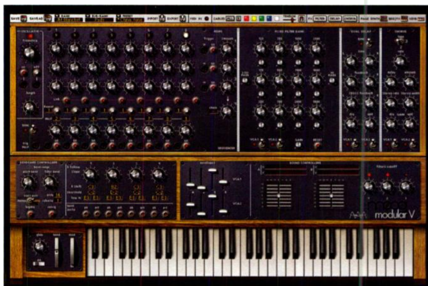
FIG. 2: The Second View control panel of Modular V contains all the keyboard and MIDI routing, the step sequencer, and the Fixed Filter Bank, Dual Delay, and Chorus effects.
