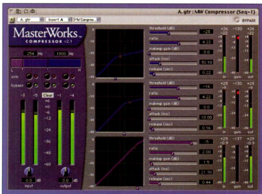
FIG. 3: MOTU's MasterWorks Compressor offers three independent bands of processing and a comprehensive feature set.
