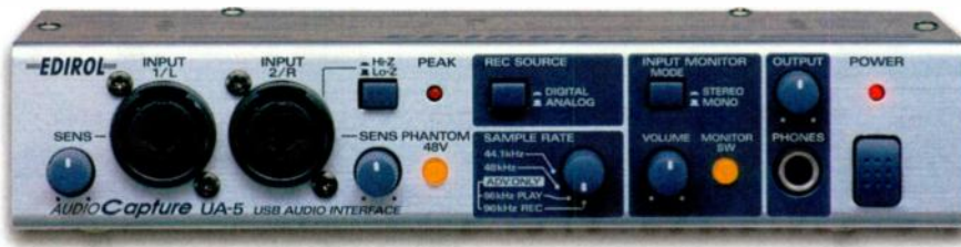
FIG. 3: The Edirol UA-5 mic pre and A/D converter can be modified for battery operation.
