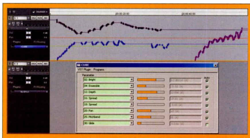
FIG. 2: The Parameter dialog provides access to as many as eight parameters at once. As you move the faders in the dialog display (bottom), automation curves appear in the track (top).
