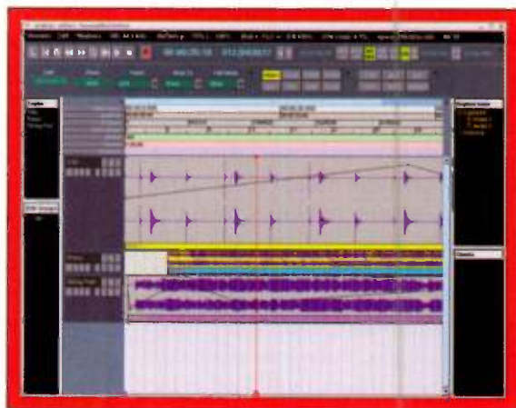
FIG. 2: Ardour is a full-featured digital audio workstation, supporting multitrack recording and mixing in an intuitive graphical environment.
