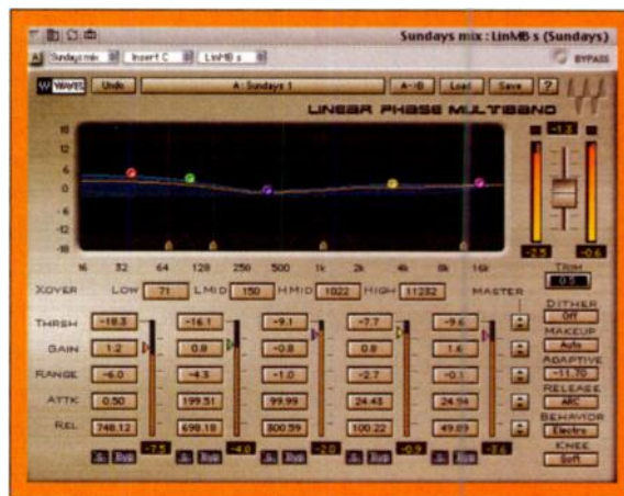
FIG. 8: Waves Linear Phase Multiband offers five independent bands of processing, ultratransparent sound, and a feature-rich interface.
