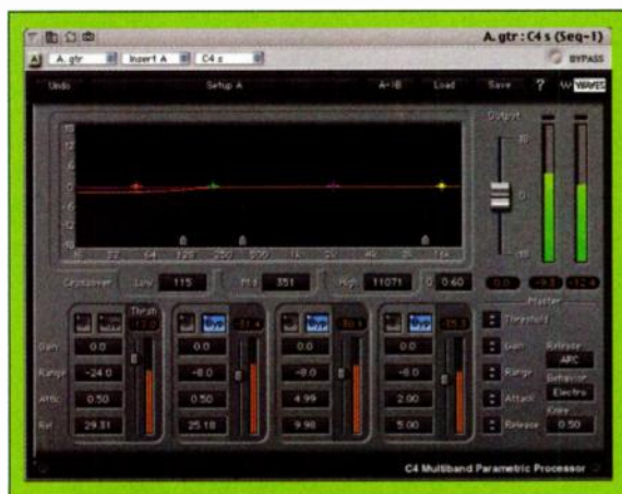
FIG. 7: Waves C4 can apply compression, expansion, limiting, and EQ in any combination (one process per band) to its independent bands.
