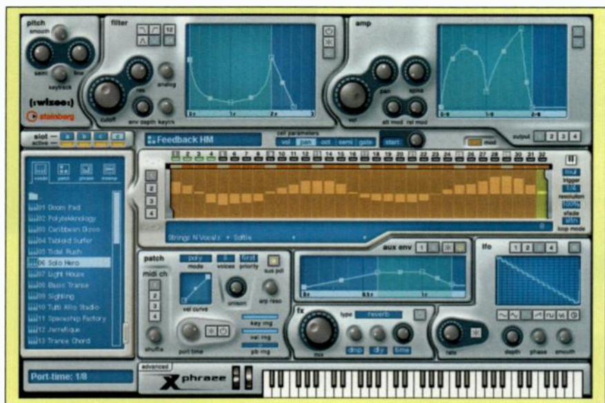
FIG. 1: Xphraze's main control panel is where you set up patches for its four independent Phraze synthesizers. The step-sequencer-style panel in the middle (called the Phraze Generator) is the sound source that is processed by the surrounding subtractive-synth modules.
