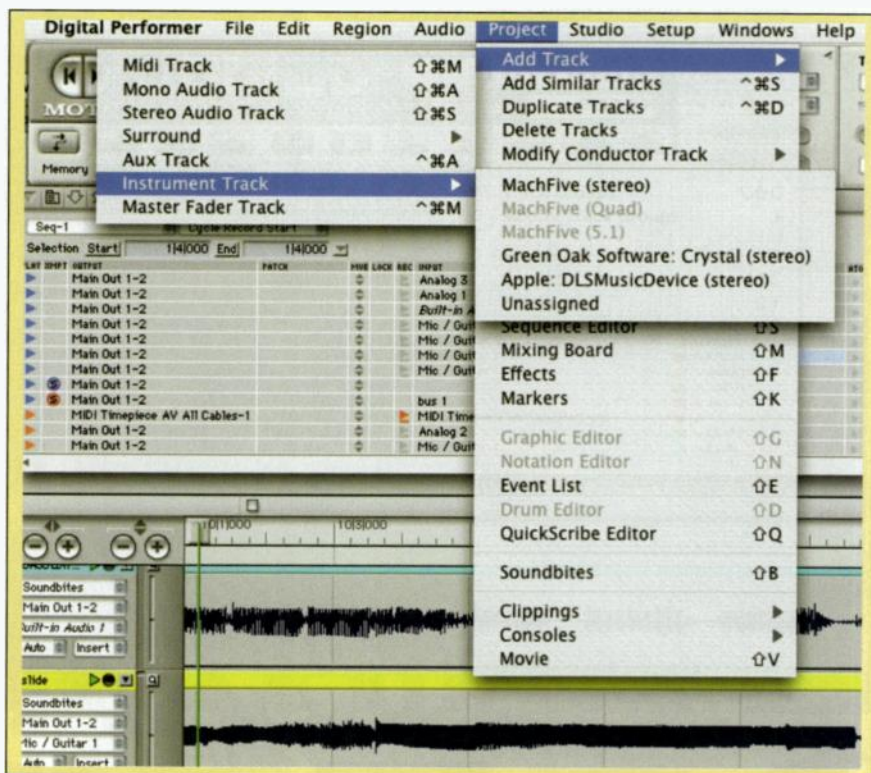
FIG. 2: One of DP4's most useful features is the Project Menu's Instrument Track option, which allows you to quickly set up virtual instruments.
