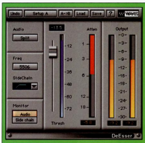
FIG. 3: A de-esser is a frequency-dependent compressor that can tame excess sibilance. Pictured here is the Waves DeEsser plug-in.
