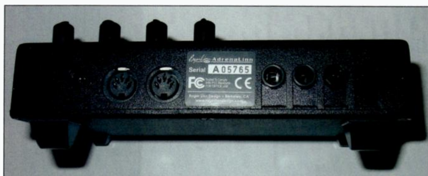
FIG. 2: The AdrenaLinn II's uncluttered back panel has a single analog input, two analog outputs, a stereo headphone jack, two MIDI ports, and a wall-wart connection.
