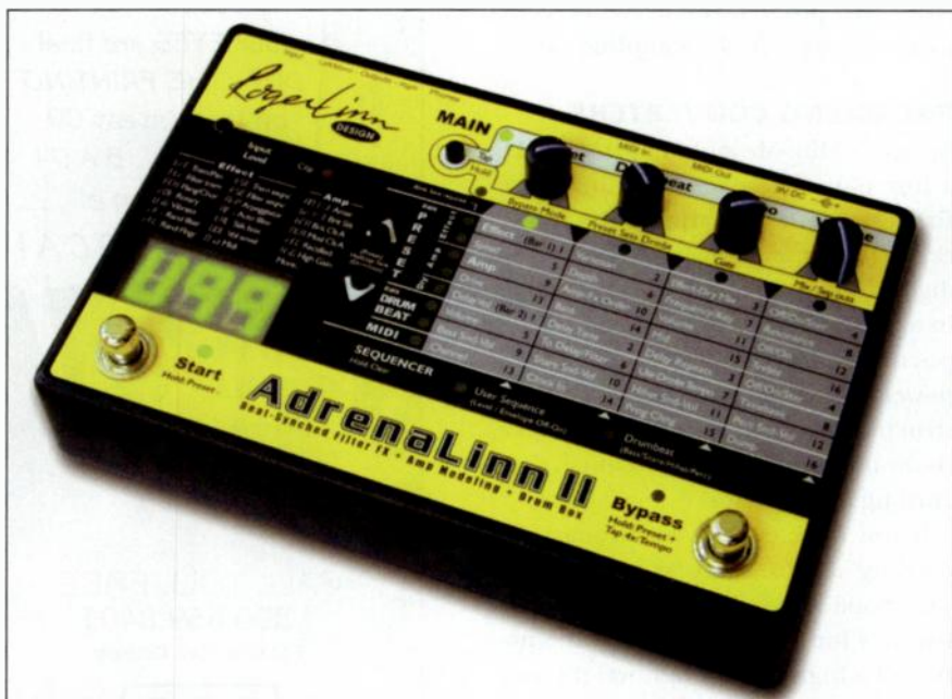
FIG. 1: Roger Linn Design's AdrenaLinn II supplies so many effects that it takes the place of several stompboxes. It also works as a basic drum machine and offers filter effects other devices can't.
