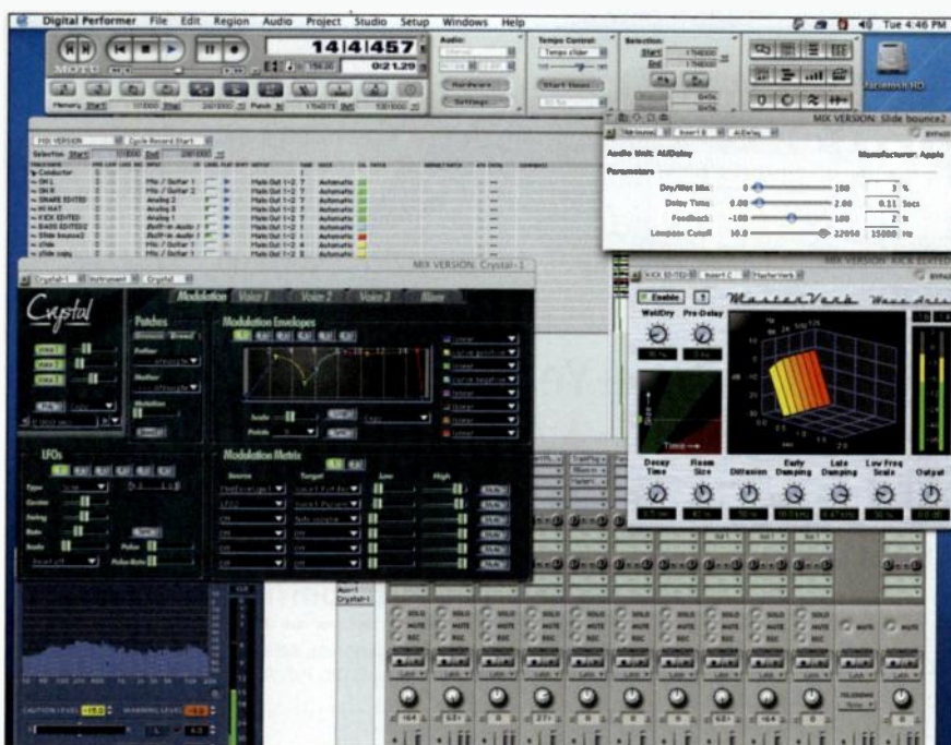
FIG. 3: Digital Performer 4.11's support of Apple's Audio Units makes it possible to access a wide range of virtual instruments and plug-ins.
