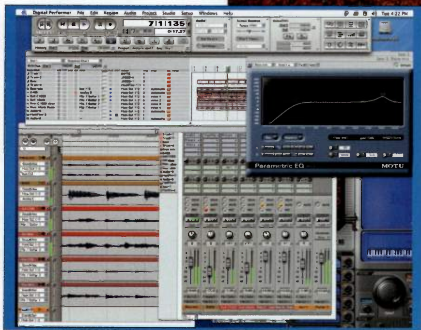
FIG. 1: The look of Digital Performer 4 is similar to that of version 3, but a new menu structure makes the program even more user-friendly and intuitive.
