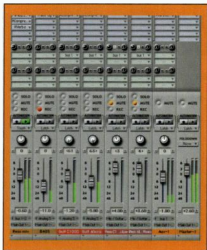
FIG. 4: The Mixing Board window now has pull-down input- and output-assignment menus (located just below the faders) for each track.
