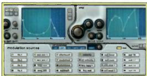
FIG. 3: Xphraze's modulation matrix lets you route a variety of sources, including built-in envelopes, LFOs, and MIDI controllers, to modulate virtually any synthesis parameter. You can route a single source to multiple destinations with different polarities and amounts.
