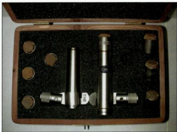
FIG. 1: The T.H.E. microphone system lets you combine a KA-04 preamp with a number of large- and small-diaphragm capsules. This set includes cardioid, hypercardioid, diffuse-field omni, and free-field omni small-diaphragm capsules.
