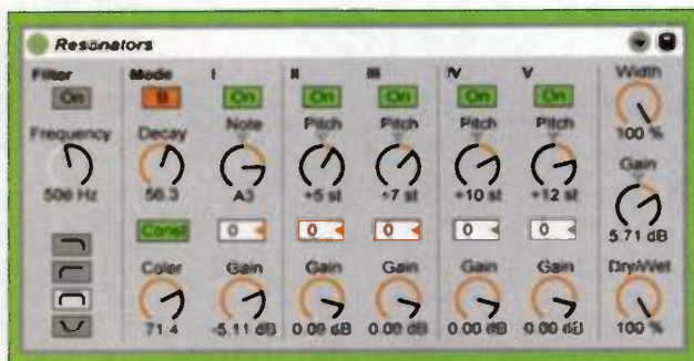
FIG. 3: The Resonators effect applies five resonators to the incoming signal. The first determines the base pitch and applies to both stereo channels. The remaining four resonators are tuned relative to the first and apply alternately to the left and right channels.
