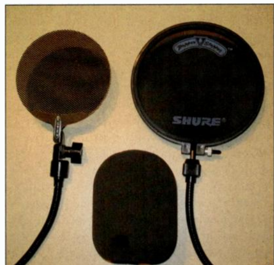
FIG. 4: To reduce plosives, you can use a metal pop filter (left), a foam windscreen (or "sock," center), or a mesh pop filter (right). Pop filters are better in most situations because they don't attenuate highs as much as foam screens do.
