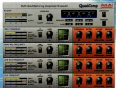
The QUADCOMP is a multi-band compressor/expander that can be used for mastering purposes.
