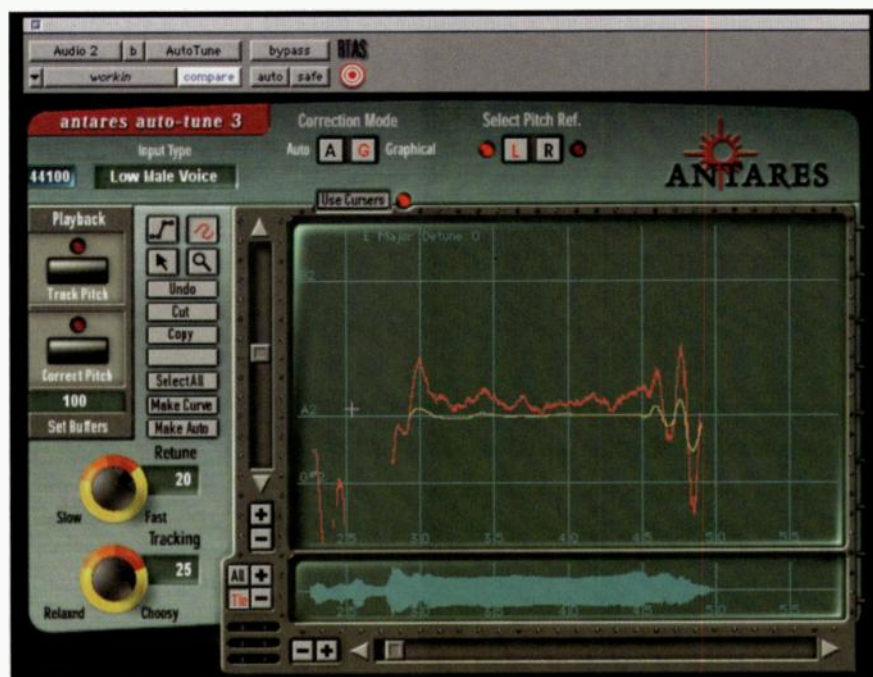
FIG. 4: This screen shot shows Antares Auto-Tune in Graphical mode. A section of the vocal track was selected and then analyzed by Auto-Tune. The resulting waveform appears in red and is clearly sharp. The yellow line represents the hand-drawn correction, and it still maintains some of the vibrato of the original note.
