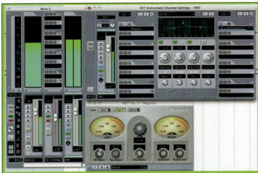
FIG. 2: The mixer here displays channel strips for a MIDI track (left), a DSP effect track (center), and a VSTi track (right). The Channel Settings window for the VSTi track appears at top right above the control panel for the new Magneto tape-simulation plug-in inserted into that track.
