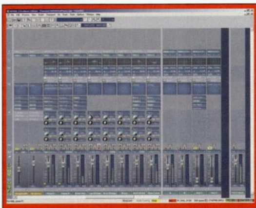
FIG. 2: Sonar's Console view has customizable channel strips, EQ available on every track and bus, graphical EQ plots, and easy access to plug-in effects parameters.
