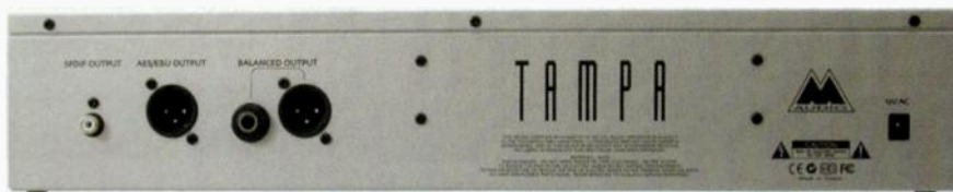
FIG. 2: The rear panel includes 24-bit S/PDIF and AES/EBU dual-mono digital outputs.
