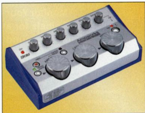
The Ampworks modeling processor is less than six inches wide and weighs less than half a pound.
