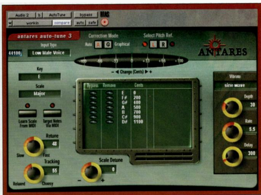
FIG. 2: Here, the Antares Auto-Tune plug-in is set to correct to an E-major scale in Auto mode. The Retune and Tracking controls are set about half way, which is a good setting when only mild correction is needed.
