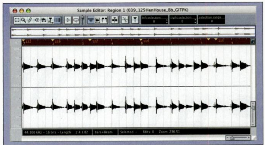
FIG. 3: By inserting tempo changes in the Tempo Track as you drag a beat position to a time position in an audio or video file, the Time Warp Tool allows you to align time positions with bar and beat locations. Here the yellow wedges indicate beat positions that have been dragged to hits in the guitar audio track.
