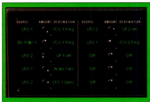
FIG. 2: For each Preset, CS-80V's modulation matrix allows ten mappings of control sources to synthesis parameters.
