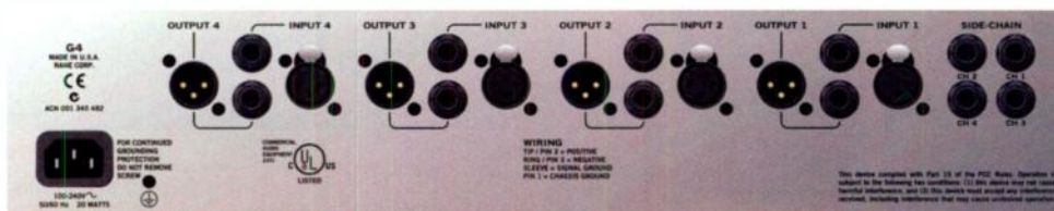
FIG. 2: The back panel of the G4 has four \frac{1}{4} -inch TRS sidechain inputs and XLR and balanced \frac{1}{4} -inch TRS inputs and outputs for each of the four channels.
