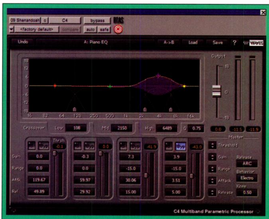
FIG. 1: The C4 Multiband Parametric Equalizer offers four bands of dynamic equalization. The third band, between the Mid and High crossover settings, applies the boost indicated by the yellow bell-shaped curve as long as the signal level in that band remains below the Threshold setting. As the signal level exceeds the threshold, the EQ curve changes shape as indicated by the shaded region.
