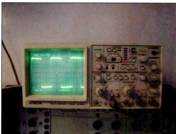
FIG. 1: An oscilloscope displays a time-domain view of a waveform.
