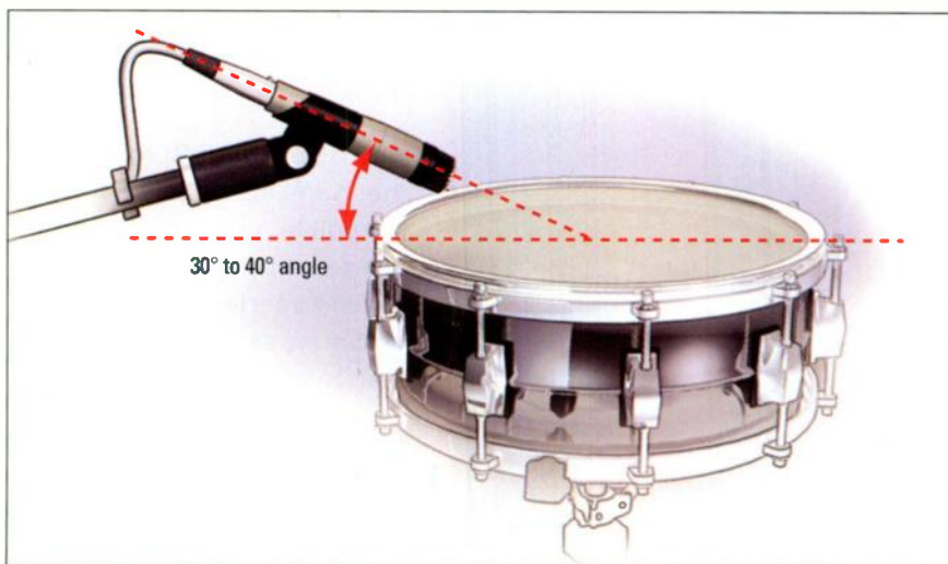
FIG. 4: The sound that the snare mic picks up will be determined not only by the particular drum and mic, but also by where the mic is aimed, its angle, and how close it is to the drum. Start with the mic cap two inches above the head, angled 30 or 40 degrees, and aimed just shy of center.
