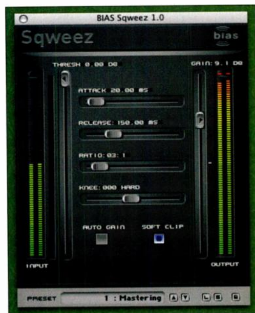
FIG. 3: Peak 4.1 includes Squeeze, a high-quality VST compressor/limiter plug-in with 14 presets, covering a range of applications.
