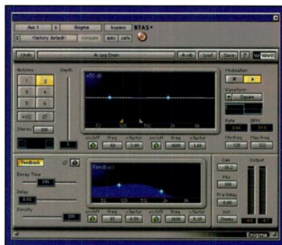
FIG. 4: Enigma is a feedback resonator effect based on notch filtering. The setup shown here turns a standard drum kit into a percussion kit with sound like a log-drum.
