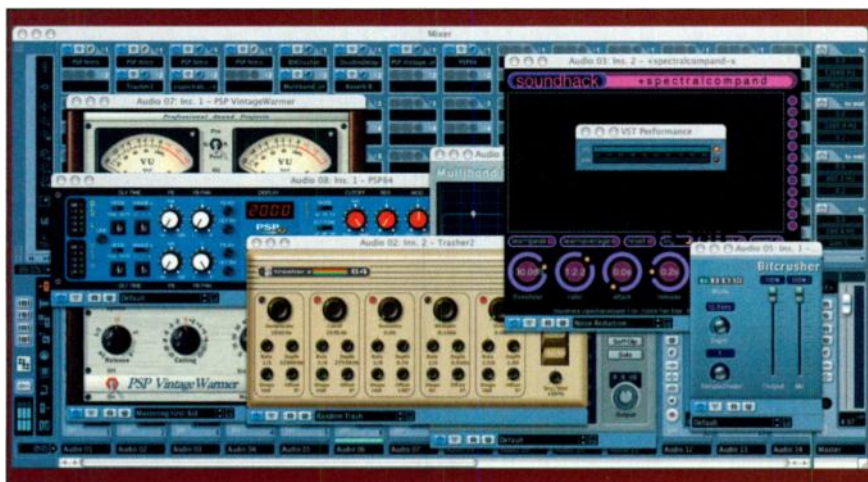
FIG. 3: Effects can put a strain on the CPU. Shown above, 12 insert effects plug-ins have pegged Cubase's System Performance meter. Printing the effects by bouncing the tracks alleviates the problem.
