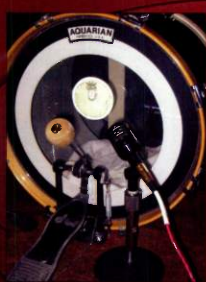
FIG. B: For a quick alternative to removing the front head on a kick that's just too boomy, mic the drum from behind with the diaphragm aimed at the beater-strike area.
