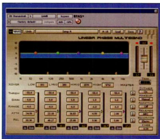
FIG. 2: Linear Phase Multiband has five bands of dynamic equalization with phase-linear crossover between bands. Its linear response makes it an ideal tool for applying dynamic EQ to some bands while leaving others untouched.
