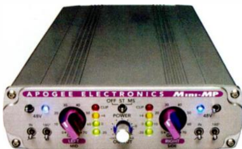
The ½-rackspace Mini-MP mic preamp features two channels, each with phantom power, highpass filter, and phase reversal switch.
