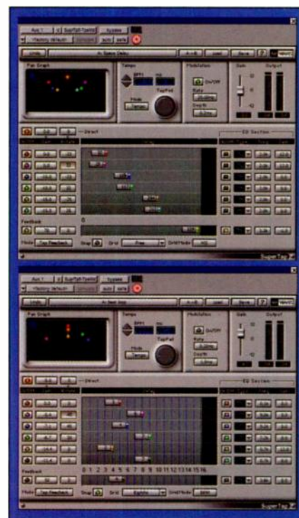
FIG. 3: SuperTap is a 6-tap feedback delay line. Its delays can be synchronized to tempo and set in note-value increments or can be free running and set in milliseconds. The top setup shown here adds space around a vocal or lead instrument. The bottom setup, synched to tempo, fills out a drum loop with new beats.
