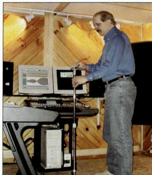
FIG. 2: Acoustician Doug Ferrara prepares to measure the response of a typical project studio's control room.
