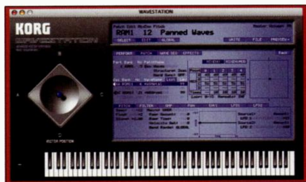
FIG. 3: Wavestation's Patch Edit page provides access to oscillators, filters, envelope generators, and various other basic building blocks of vector synthesis.
