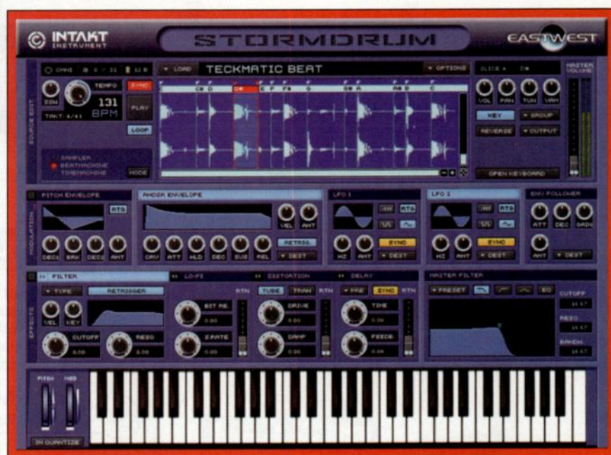
FIG. 2: The interface of Quantum Leap Stormdrum , based on Native Instruments' Intakt sampler, enables access to sound-shaping tools such as a multimode filter, envelope follower, two LFOs, and effects.
