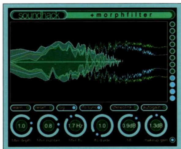
FIG. 2: +morphfilter morphs between two 513-band filters that can be drawn in manually with a mouse or captured by analyzing incoming audio. You can control the morphing by a tempo-synchronized LFO, by incoming MIDI, or manually.
