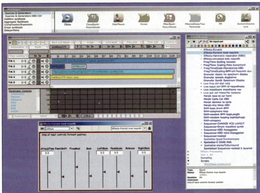
FIG. 2: Kyma has several dedicated work areas that are suited to a variety of tasks. The Sound Browser allows access to all the examples that come with the system.
