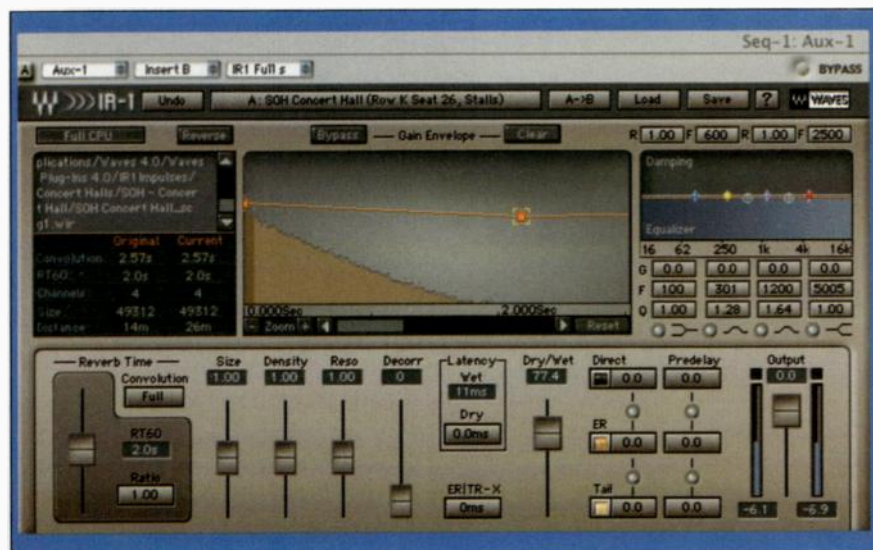
FIG. 5: Waves IR-1 is the only convolution plug-in that supports both Mac and Windows. It also has the distinction of providing the most complete control of traditional reverb parameters such as size, density, and pre-delay.
