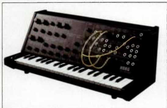
FIG. 5: Although the MS-20iC looks just like a slightly smaller version of the original MS-20 synthesizer, it is a USB keyboard and control surface that is handy to use with almost any soft synthesizer.
