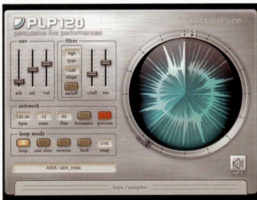
FIG. 1: The radarlike "loop eye" in Best Service's PLP120 Percussive Live Performances interface has a visual representation of a loop and dials for changing its start and end points.
