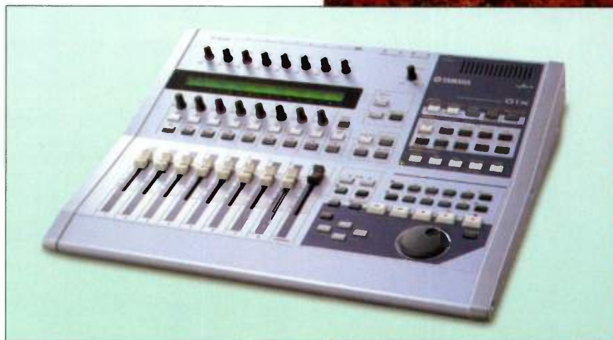
FIG. 1: The Yamaha 01X combines the functionality of a freestanding digital mixer, two effects processors, a DAW control surface, and an mLAN-based audio and MIDI interface in a single device weighing less than 14 pounds. Impressive flexibility and outstanding ergonomics ensure ease of operation.
