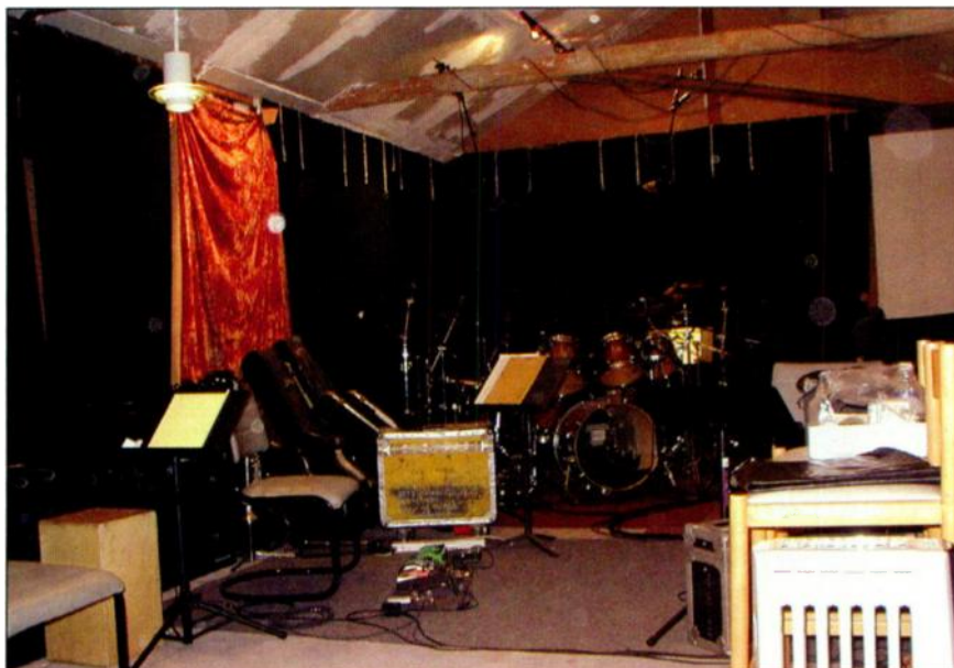
FIG. 7: This view inside of the Barn shows the boom arms that were attached to rafters to hold the Audio Technica AT4060s used for overheads.
