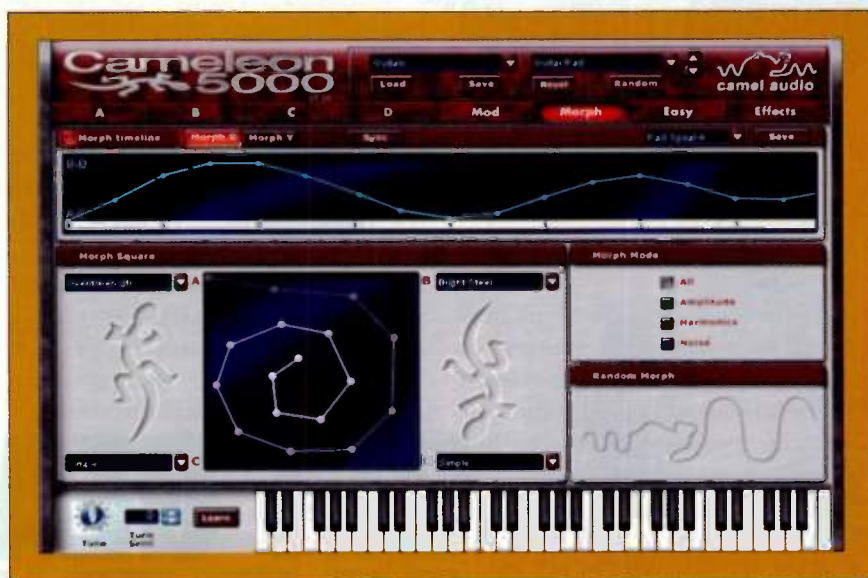
FIG. 2: The corners of Morph Square represent Cameleon's four voices. The dot-and-line graphic within the square represents the morphing pattern among the four voices. The Morph Timeline at the top shows the horizontal (Morph X) or vertical (Morph Y) morphing pattern over time.
