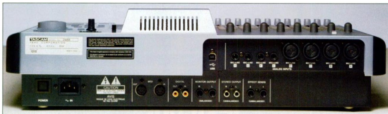
FIG. 2: With the exception of a dedicated guitar-and-bass input, a headphone out, and punch-in/out and expression-pedal inputs on the front of the unit, the 2488's connections—including line and mic inputs, main and monitor analog I/O, digital I/O, and MIDI I/O—are located on the rear panel.
