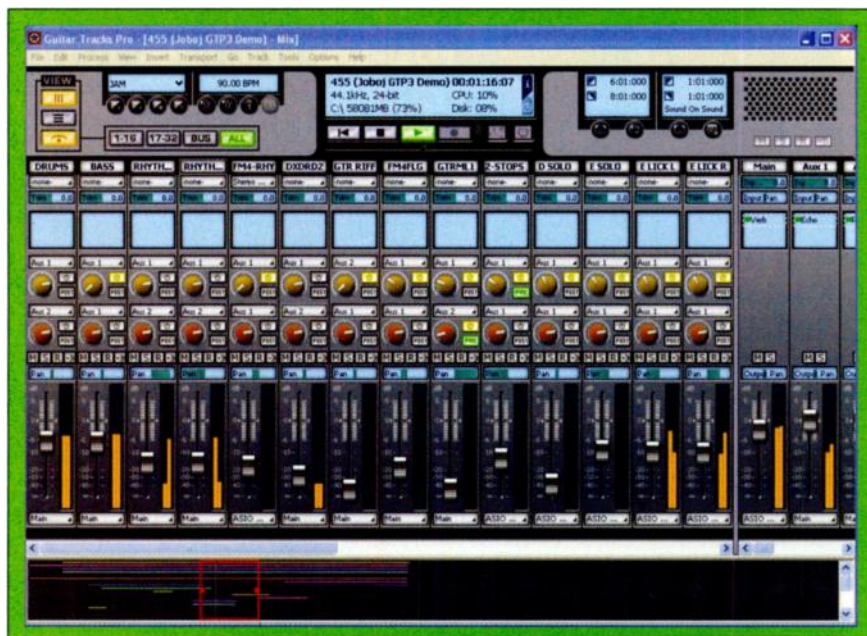
FIG. 1: Cakewalk Guitar Track Pro 3's Mix view offers a fully featured and familiar-looking mixing console that displays 32 audio channels, 8 buses, and 2 aux buses.
