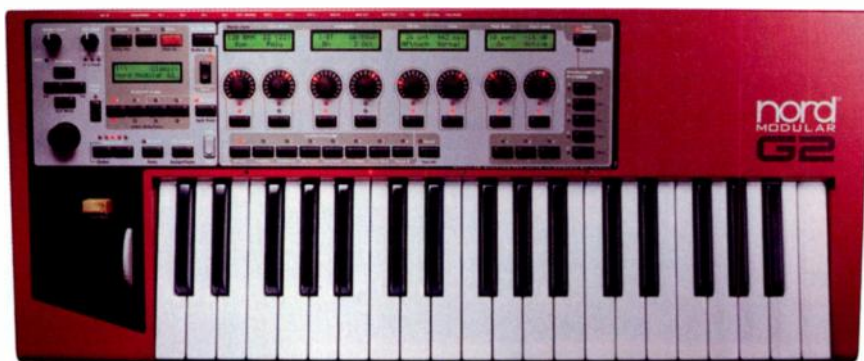
FIG. 1: Clavia's new Nord Modular G2 expands on its predecessors by offering more horsepower and new modules. The system is available in several configurations, including three- and five-octave keyboards and a rack unit.
