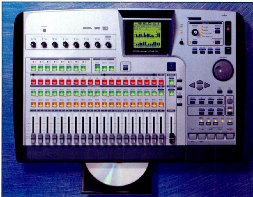
FIG. 1: The Tascam 2488 has 24 tracks of uncompressed digital recording, lots of effects, a GM tone module, a CD-RW drive, a USB 2.0 port, a 40 GB hard drive, and more—all for a surprisingly low price.
