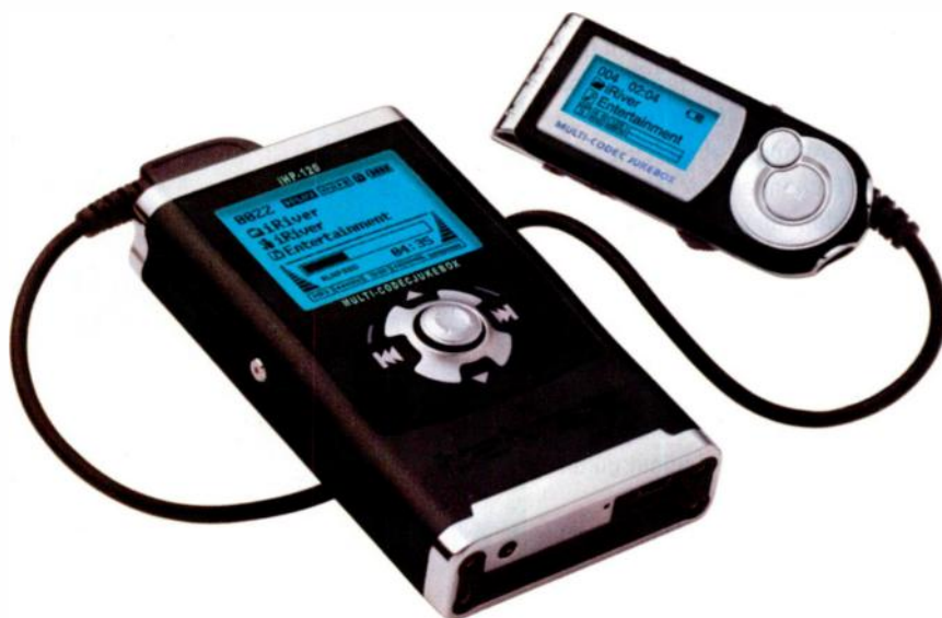
The iRiver H120 is an MP3 player that can record 16-bit, 44.1 kHz uncompressed WAV files.
