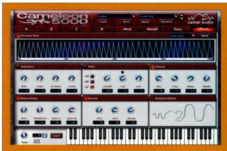
FIG. 3: Cameleon's Effects panel offers standard distortion, chorus, stereo delay, and reverb as well as multiband and formant filtering. The formant filter's spectrum is controlled with a breakpoint display (top) offering as many as 128 breakpoints.
