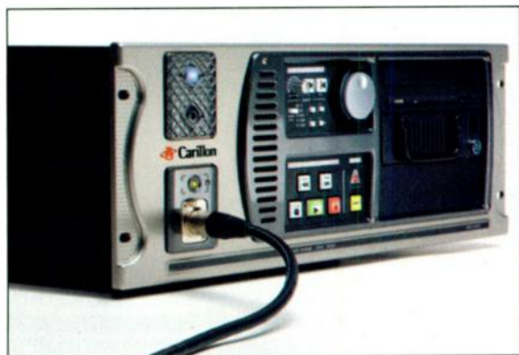
FIG. 2: Carillon's unique rackmount (4U) case is designed to be especially quiet. Extra features such as the transport controls and Neutrik connector add to its convenience.
