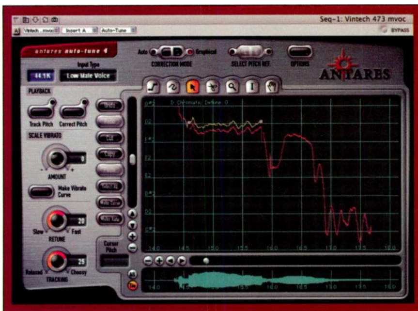
FIG. 2: Auto-Tune 4's Graphical mode includes useful new tools for the Pitch graph and the Envelope graph, and a better-organized layout of navigation controls.
