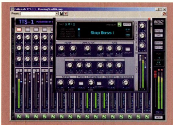
FIG. 3: The TTS-1 soft synth has a full set of General MIDI 2 patches that sound great. Patches can be edited, and settings can be automated using MIDI continuous controllers.
