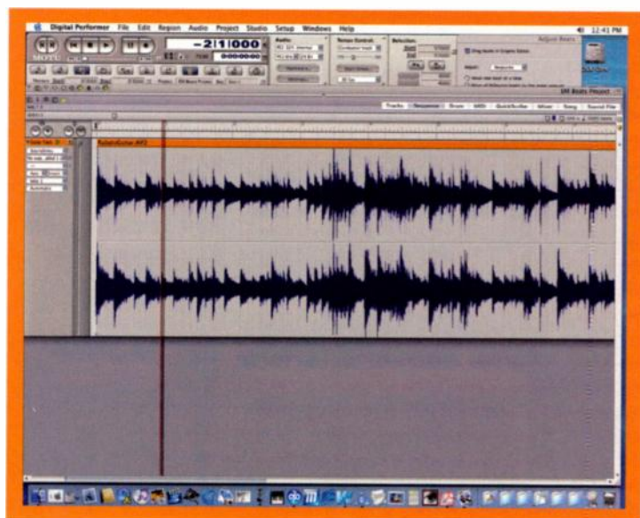
FIG. 2: With Adjust Beats you can align the time ruler's bar and beat marks by dragging them over peaks in audio waveforms.
