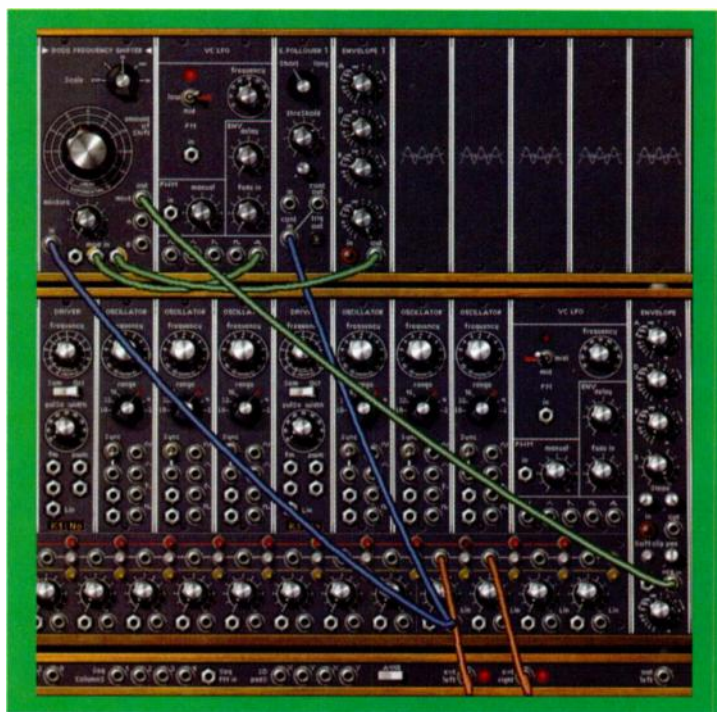
FIG. 1: The frequency shifter setup for toms uses an envelope follower to trigger a standard ADSR envelope, which is used to modulate the amount of frequency shift. The envelope's release time controls the contour of the modulation.
