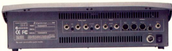
FIG. 2: The Command|8 rear panel includes audio and MIDI I/O jacks as well as USB and footswitch input jacks.
