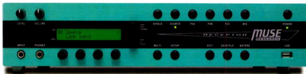
FIG. 1: Receptor's front panel features a 2-line, 48-character backlit LCD display; four freely assignable rotary encoders; a guitar input; a headphone output; and buttons for fast access to important functions.
