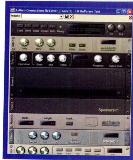
FIG. 1: Alien Connections' ReValver lets you create a guitar amp from its virtual Modules.
