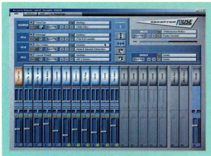
FIG. 5: Muse Control software provides a graphic user interface for programming Receptor's mixer as well as individual plug-ins that use their own graphic user interfaces.
