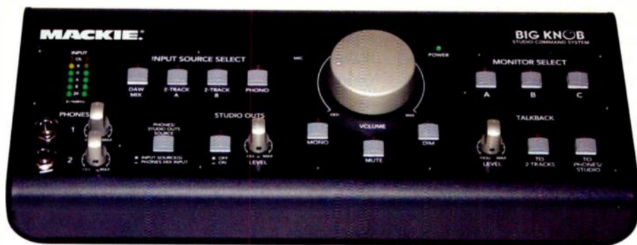
FIG. 1: Big Knob, which offers DAW users the functionality of a console monitoring section, draws its name from the massive volume knob that sits in its center.
