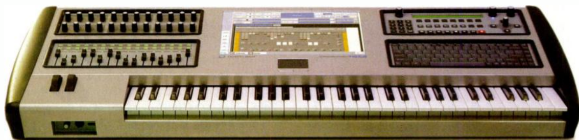
FIG. 1: The OpenSynth neKo 64 combines a powerful Windows XP computer running virtual instruments or your favorite audio applications with a gig-worthy keyboard and numerous MIDI controls for real-time tweaking.
