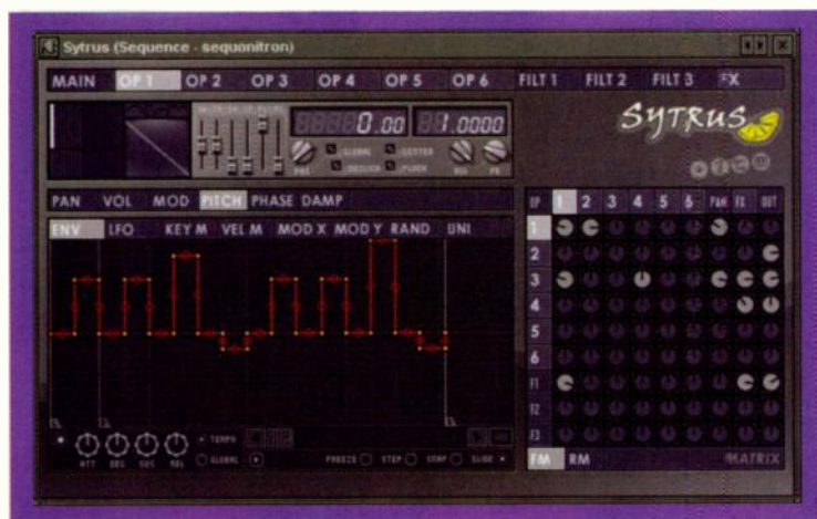
FIG. 2: The 6-operator Sytrus synth has multisegment envelopes (lower left). FM and RM amounts are programmed in the knob matrix at right.
