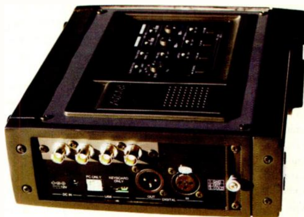
FIG. 2: The FR-2's left side panel provides digital audio ins and outs, including two USB ports and XLR I/O that can be configured as S/PDIF or AES/EBU. The BCN connectors are for the time-code option.
