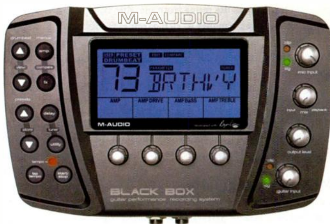
FIG. 1: The Black Box combines a USB recording interface with an AdrenaLinn-inspired guitar-modeling and sequenced-effects processor, as well as a drum machine.
