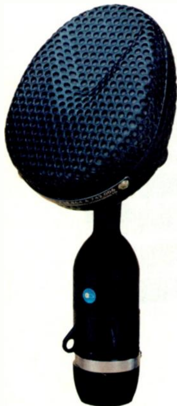
FIG. 3: The Coles 4038 has been a studio staple for decades. It covers everything from drum overheads and brass instruments to woodwinds and strings with equal aplomb
