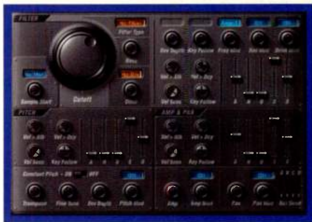
FIG. 2: MOTU's MachFive follows its sample-playback engine with the standard subtractive-synthesis signal path consisting of a filter, amplifier, and two ADSR envelope generators for modulation.
