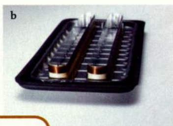
FIG. 1: The MRS diaphragm includes ribs and notches (gussets) to minimize breakup modes (a). Two elongated voice coils apply uniform force to the entire surface (b).
