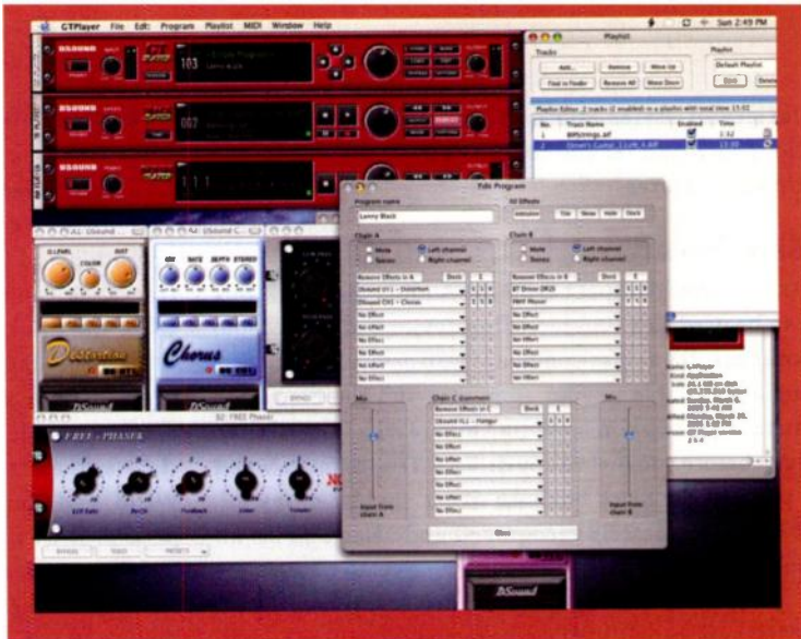
FIG. 1: GT Player offers guitarists plenty of options for processing live guitar, for playing live ReWire and audio-file accompaniment, and for making use of MIDI control.
