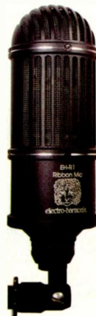
FIG. 8: The Russian-made Electro-Harmonix EH-R1 is an updated version of the Oktava ML-52. It has a dip in the frequency response at 7 kHz, which contributes to its relatively dark sound quality.
