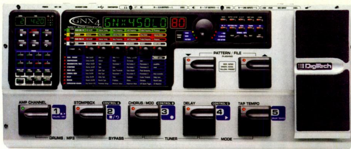
FIG. 1: In addition to its modeling and multi-effects functions, the DigiTech GNX4 is an 8-track recorder, a USB MIDI and audio interface, a mic preamp, a looping device, and much more.
