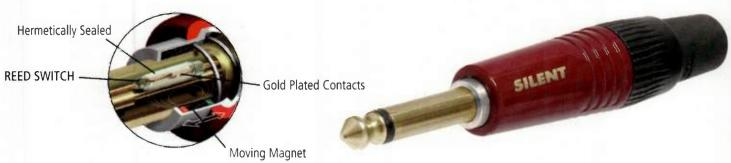
Introducing NP2C-AU-SILENT - the new "silent plug" from Neutrik. With a built-in reed switch that mutes pops and squeals. The unique plug design resists dust and dirt, so the reed doesn't corrode, there's no wear and tear on the contacts - and lifetime is virtually unlimited. Look for the distinctive red plug with "silent" on the shell. Make grandma happy.
