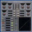
Modeled from the extremely flexible OXF-R3 dynamics processor, it features Mono and Stereo Channel Dynamics with separately controlled sections for Compressor, Limiter, Expander, Gate, 2 Band Side-Chain EQ and 'Warmth' feature. Also includes 6 **Channel Bus Compressor.**
