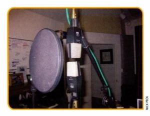
FIG. 3: Any two mics can be used for mid-side recording, as long as they have the appropriate polar patterns.
