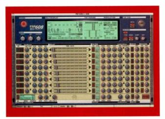
Controls for each of the PSP 608's taps are identical, and the LCD-style display at the top annotates the settings when the mouse passes over a control.
