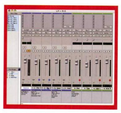
FIG. 5: An example DAW mixer set up to separate a finished left/right mix into M-S, adjust levels, and decode back to left/right. The Trim plug-ins are used for polarity reversal.
