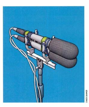
FIG. 2: Typically, directional and bidirectional mics are placed on top of each other for M-S recording.
