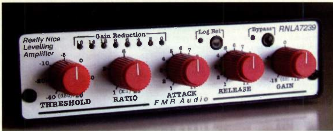
FMR Audio's Really Nice Levelling Amplifier uses a gain element that gives the unit a distinct sonic character.
