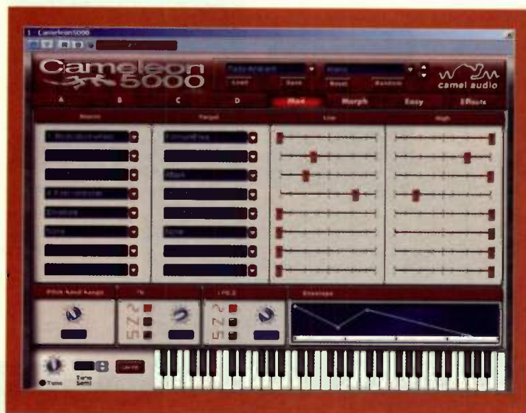
FIG. 2: The modulation matrix in Camel Audio Cameleon 5000 has minimum- and maximum-amount sliders. Here, the High setting is lower than the Low setting for the fourth routing, so the modulation will be inverted.
