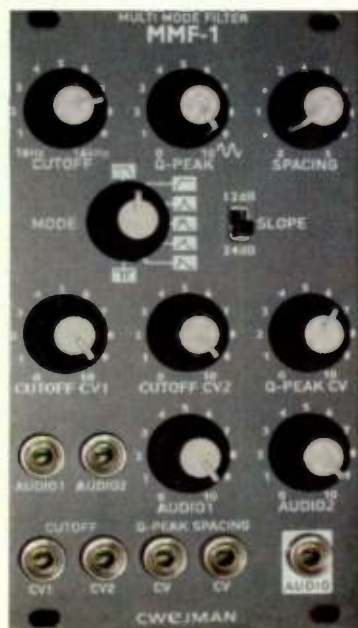
FIG. 5: The Cwejman MMF-1 multimode filter offers three dual bandpass modes, each of which gives you two sine tones when the filter goes into resonance.
