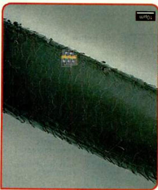
FIG. 1: IBM's nanotube-based ring oscillator is one-fifth the width of a human hair.
