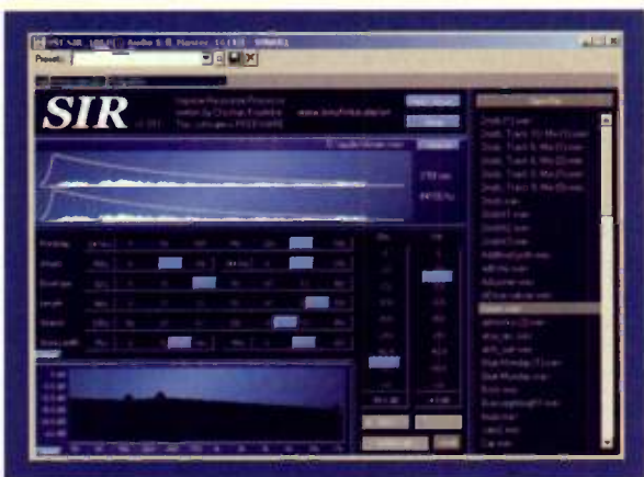
FIG. 1: Christian Knufinke's free SIR Impulse Response Processor runs as a VST effects plug-in and can use any WAV file as an impulse response. You can alter the IR in a variety of ways before it is applied to an audio file.
