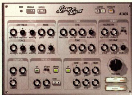
FIG. 1: The Lounge Lizard EP-3 control panel B houses the physical-model controls, which have been slightly expanded and rearranged.
