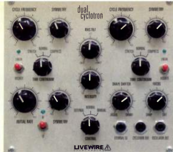
FIG. 3: In the Livewire Dual Cyclotron, three oscillators interact with each other, sometimes in seemingly mysterious ways.
