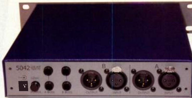
FIG. 2: Bus jacks on the 5042's rear panel accommodate interconnection with other modules in Rupert Neve Designs' Portico Series.
