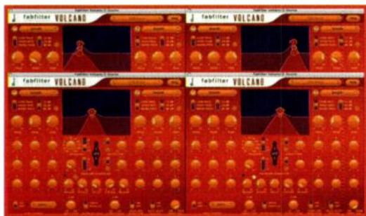
FIG. 1: Four instances of Volcano are set up as modulated notch filters, then arranged in series for a simulated flanging effect.
