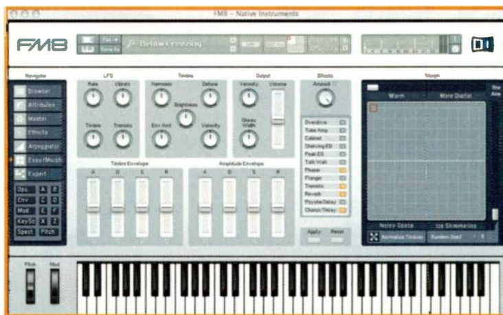
FIG. 3: The Easy/Morph page greatly simplifies the FM sound-design process. The large Morph controller on the right is replicated in a smaller one at the top of all pages.
