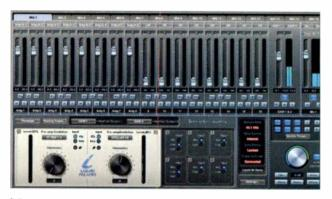
FIG. 3: A software-controlled, DSP-based mixer on the Saffire allows any 18 channels to be routed to any of 16 output channels with zero latency. It can also fold two channels back to the DAW.
