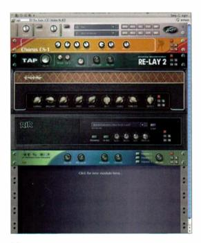
FIG. 5: The GUI for Peavey ReValver MKIII stacks modules from top to bottom in the order of signal flow.
