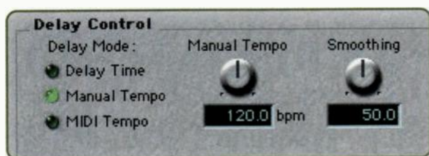
FIG. 3: Interpolated delays let you change delay times smoothly, often creating an interesting pitch-bend effect during the transition. The Smoothing knob on this control panel for an Korg OASYS PCI sound card determines how long it takes to slide from one delay value to another.
