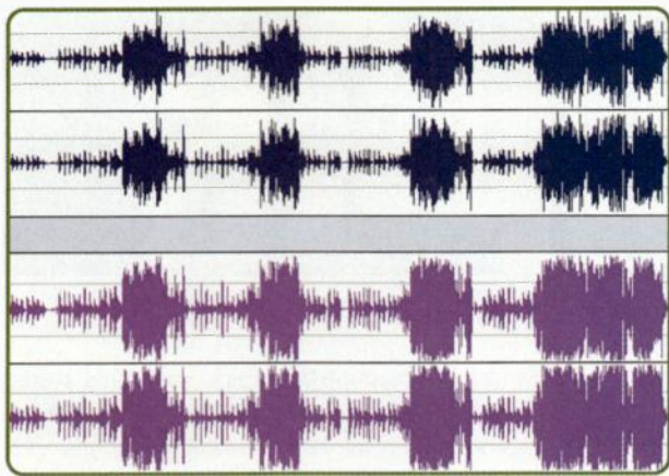
FIG. 2: The top window shows a song with uneven volume levels. The bottom shows the same file after limiting (with make-up gain); note the increased volume in the quiet passages.
