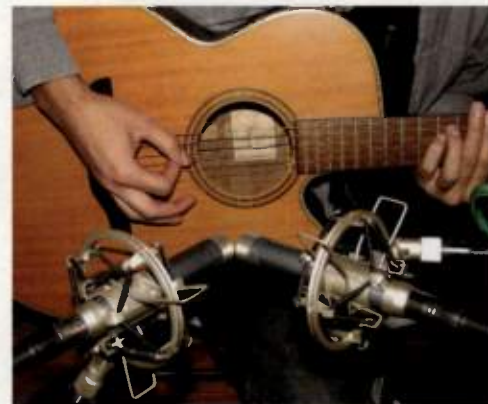
Fig. 5. X/Y miking is an option for obtaining a full-sounding stereo recording.
