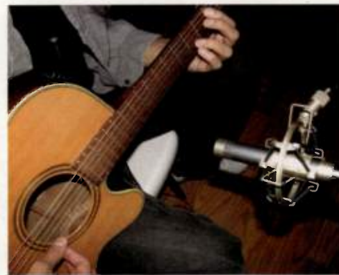
Fig. 3. Compared to stereo miking, a single microphone can eliminate the possibility of phase cancellation.
