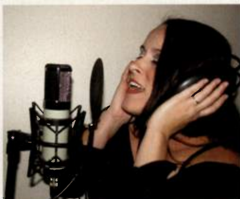
Fig. 6. A good pop filter can help reduce plosives, thus reducing the need to edit them out when mixing.
