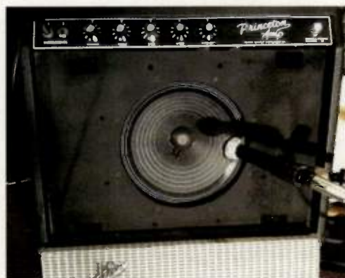
Fig. 2. Positioning the mic off-axis, and changing its angle, alters the amp's tone.
