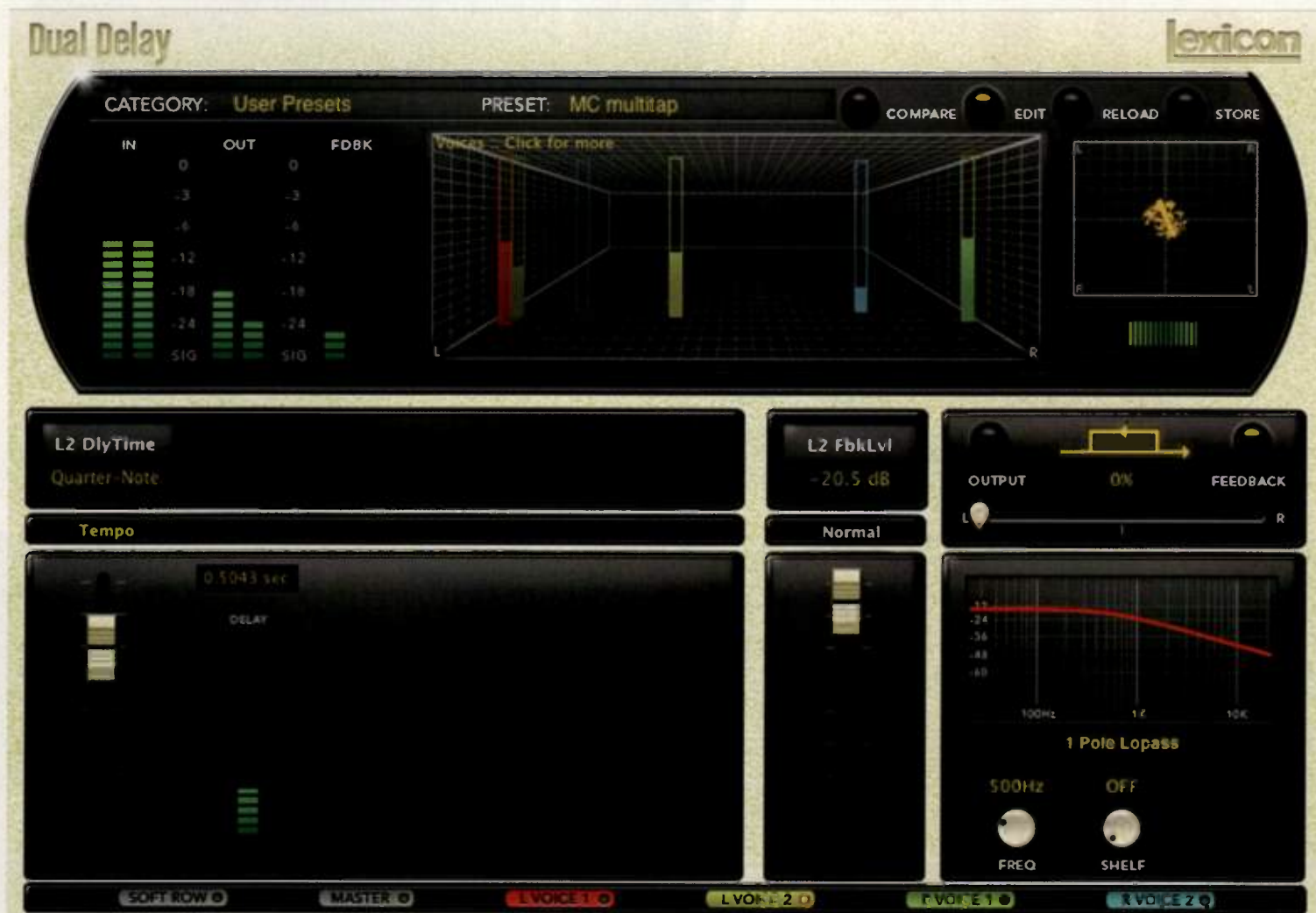
Fig. 1. Lexicon Dual Delay lets you adjust the delay time, level, panning, filtering and feedback parameters independently for each of four delay voices. In the lower-right corner of the GUI, feedback for a quarter-note delay is filtered above 500Hz, panned left and attenuated over 20dB to make it barely audible.
