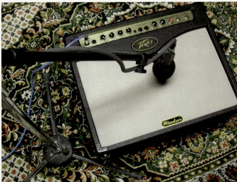
Fig. 8. If you need more low end when using an amp with electronic instruments, try turning it into a pseudo-“closed-back” cabinet.
