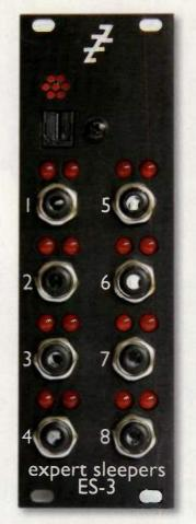
The Expert Sleepers ES-3 Mk3 is a Eurorack module that connects to your audio interface over ADAT Lightpipe so you can send CVs to your modular from your DAW.
