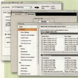
Although Echo and Roland make some ASIO interfaces that can be cascaded, you don't necessarily need a new interface. Windows itself can aggregate multiple interfaces if your software supports the WDM, WaveRT, or ASAPI driver models. (Most programs do.)
