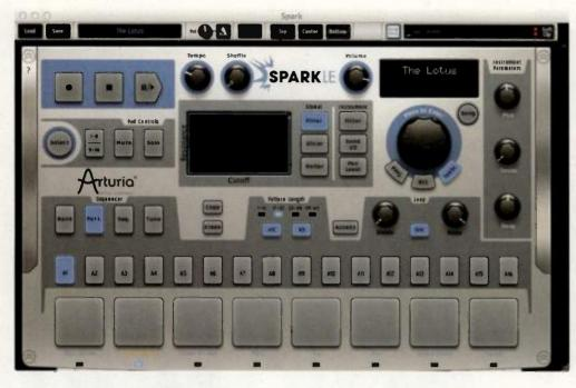
envelope, filter, and seven effects controls, allowing you to manipulate and record changes on the fly. Parameter values appear on the Spark software screen.
