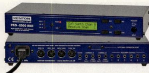
Fig. 1. The Kenton Pro-2000 MkII is a stand-alone, multichannel MIDI-to-CV converter.
