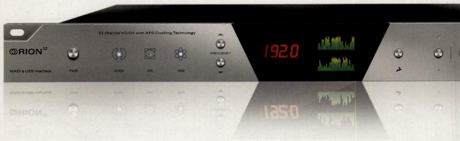
Fig. 1. Orion32 packs an impressive 32 channels of I/O, as well as a master clock, into a 1U box.
