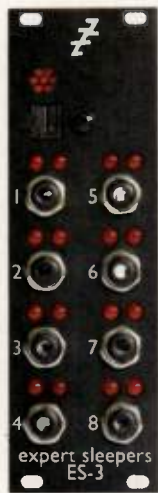
Fig. 6. The Expert Sleepers ES-3 Mk3 connects to your interface's ADAT Lightpipe port and provides 8 channels of \pm 10VDC control signals from Silent Way or similar software running on your computer. You can also send audio through any of the module jacks.
