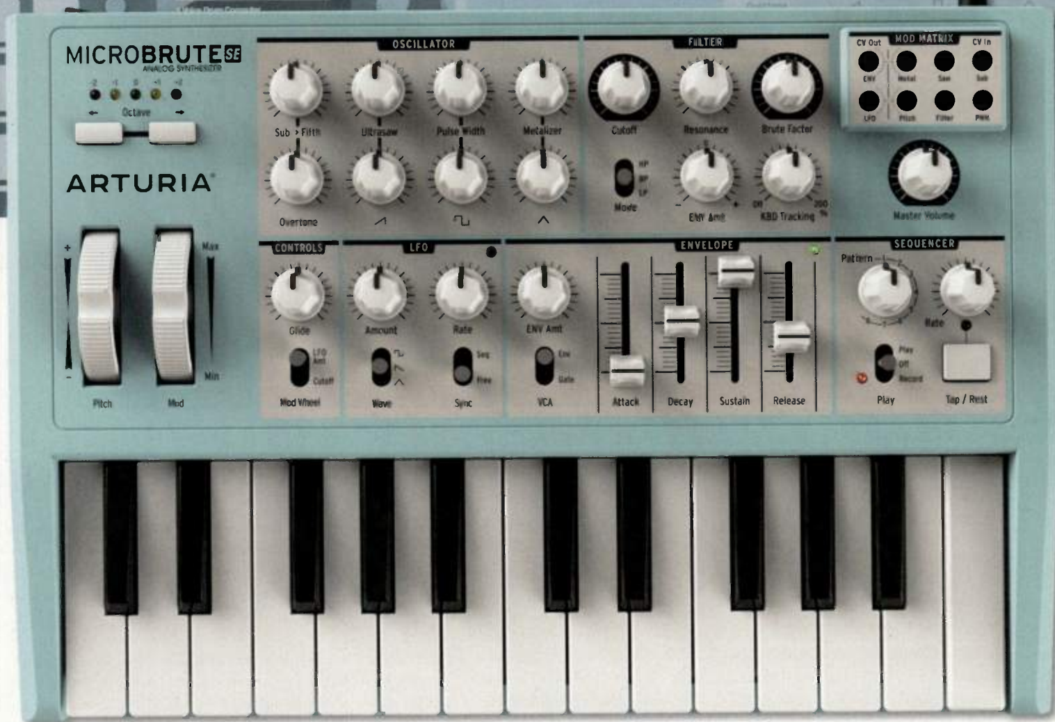
The Arturia MicroBrute SE has a built-in CV patchbay that significantly increases the modulation possibilities of the synth.
