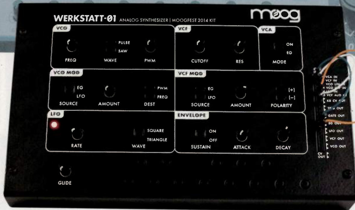
The Moog Music Werkstatt-01 is an easy-to-assemble synth kit that packs a big sound and loads of features into a small metal case.
