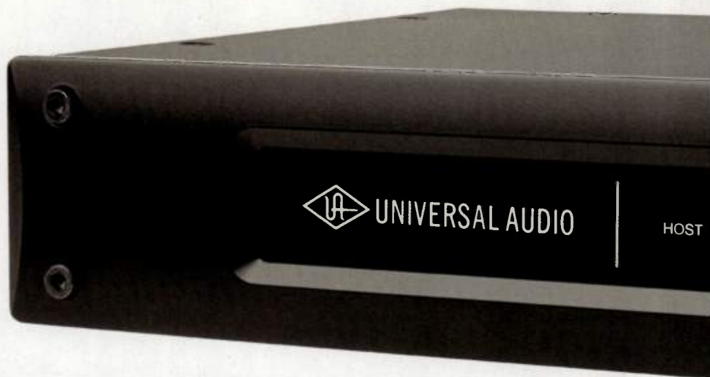
Fig. 1. The Satellite Thunderbolt allows for much higher plug-in counts than its FireWire counterparts.
