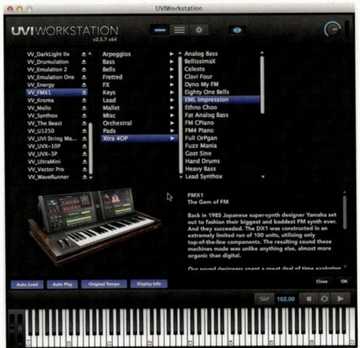
Fig. 3. Use UVIWorkstation’s browser to open libraries, instruments, and presets. Once they’re open, some instruments also have menus for selecting presets without going through the browser.
