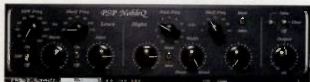
Fig. 2. The PSP NobleQ plug-in's design is loosely based on the vintage Pultec EQP-1A3 passive equalizer.
