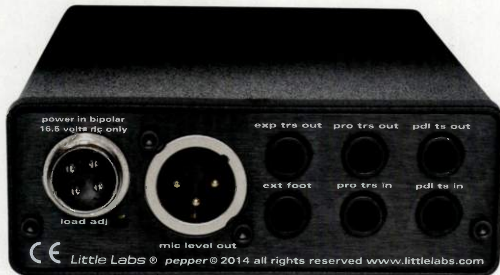
Fig. 2. Back-panel I/Os include XLR and balanced 1/4" outputs.
