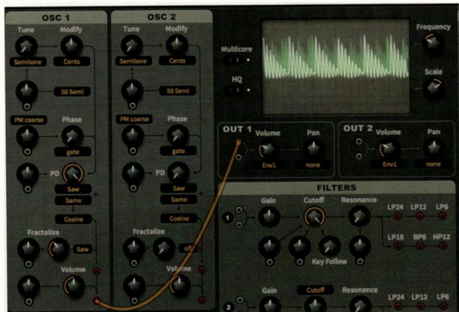
Fig. 2. A close-up of the of the Fractalize effect on a sawtooth wave. Note the repetition of the waveform in decreasing size (amplitude) within an overarching sawtooth-wave shape.
