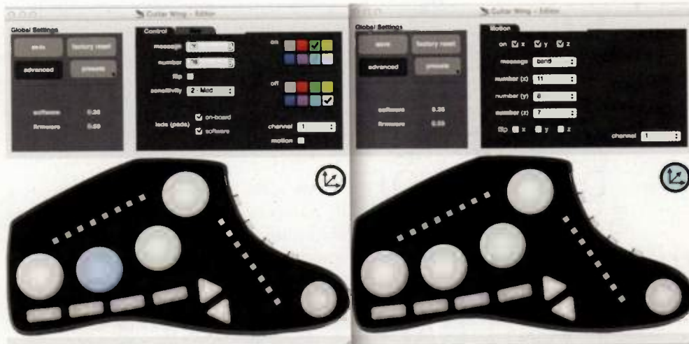
Fig. 3. I've combined two screens of the Guitar Wing Editor showing assignments for the pad, as well as setting up control using the motion sensor (indicated by a trident-like icon). Notice that each axis of the motion sensor has an independent menu.
