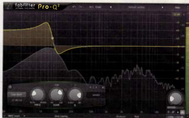
Fig. 3. A low-shelving filter's Q setting is boosted in FabFilter Pro-Q2's Zero Latency mode to create a resonant peak and dip in response below and above the filter's corner frequency, respectively.
