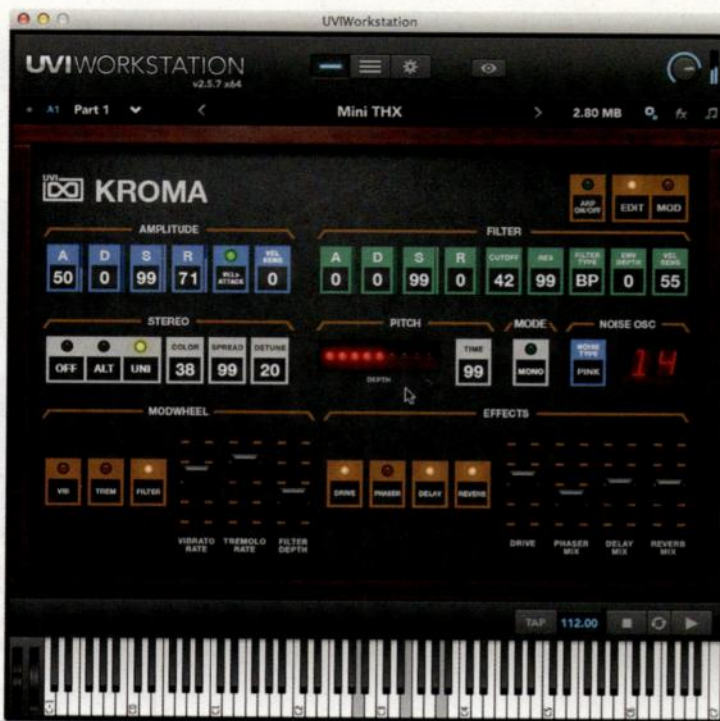
Fig. 1. Although the GUIs in Vintage Vault visually resemble the front panels of the instruments that were sampled, they all feature every parameter that UVIWorkstation makes available.
