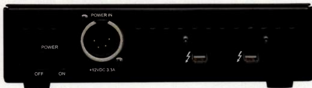
Fig. 2. The rear-panel of the unit features a power switch, power adapter input, and Thunderbolt ports.
