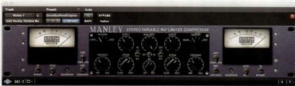
Fig. 5. The Manley Variable MU replicates the smooth sounding tube compressor and adds a wet/dry control for parallel compression.
