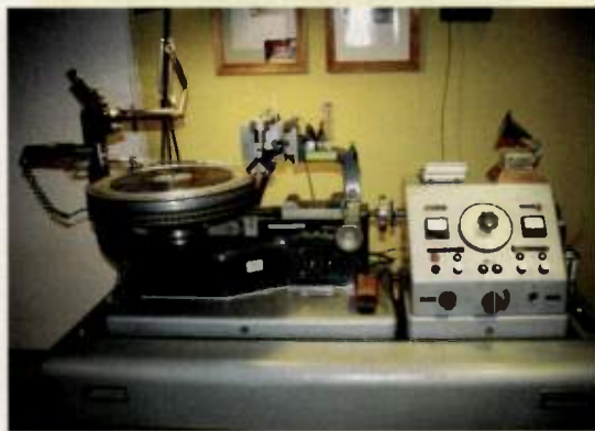
The Neumann AM-32 lathe at Infrasonic Sound, Los Angeles, CA. The large dial on the control panel on the right can be used to manually regulate the number of lines etched into the master lacquer.
