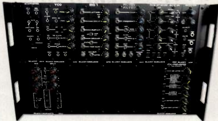
Fig. 2. The Blacet Puma 15 includes enough modules for a single MIDI-controlled synthesizer voice, with empty rack space to expand your timbral palette.
