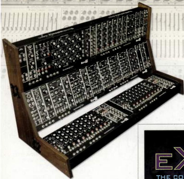
Fig. 8. The Box-66 from Synthesizers.com has walnut sides and sports six VCOs, two VCAs, four EGs, and two Moog-style sequencers, among its many modules. As with the company's other systems, you can alter the module complement in the Box-66 when you order.
