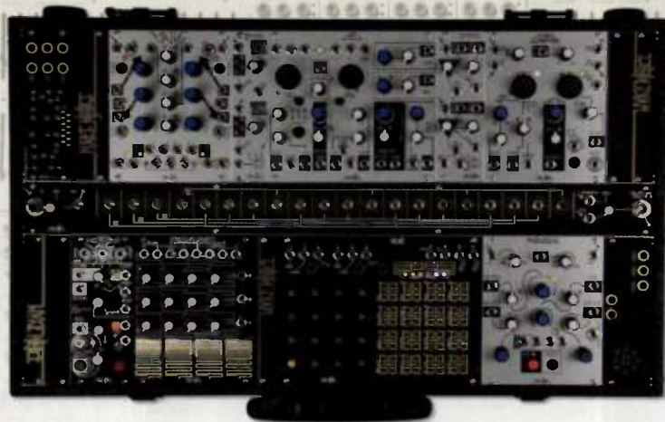
Fig. 4. The Make Noise Shared System packs a wealth of high-level functionality into a flight-friendly case.
