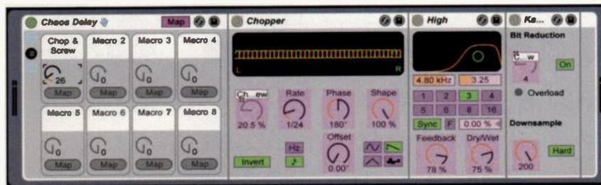
Fig. 3. Here we're routing both LFO mod amount and bit depth to one macro control.
