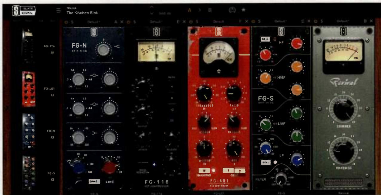
Fig. 1. Virtual Mix Rack accommodates up to eight processing modules and currently includes two compressors, two equalizers, and a sonic enhancer.
