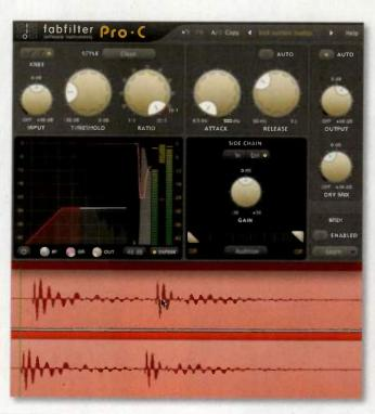
Fig. 1. A mult of a kick drum track (the mult's red waveform is the bottom one shown here) is advanced in time 2 ms with respect to the original track (shown immediately above the mult). The mult is then bused to the external sidechain input of the FabFilter Pro-C compressor inserted on the original track, effectively arming Pro-C with lookahead detection.
