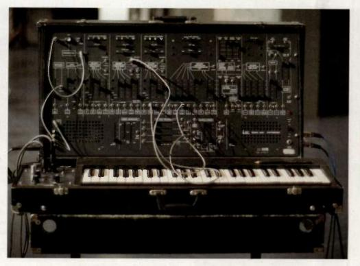
Classic synths like the ARP 2600 let you modulate the lowpass filter with an audio-rate wave, the first step in generating a talking sound.
