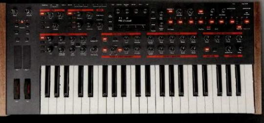
4-voice paraphonic  $\cdot$  dual analog filters  $\cdot$  4 oscillators plus sub osc  $\cdot$  32-step, multitrack sequencer 4 CV ins & outs  $\cdot$  4 LFOs  $\cdot$  5 envelopes  $\cdot$  3 digital delays plus digital BBD  $\cdot$  arpeggiator character FX  $\cdot$  16 x 2 modulation matrix  $\cdot$  analog distortion  $\cdot$  tuned feedback
