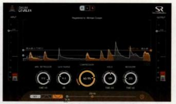
Fig. 2. Drum Leveler applies upward compression to weak hi-hat strikes. The sidechain's bandstop filter removes just enough energy from bleed to keep it out of (above or below) the processing range set by dual thresholds.
