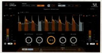
Fig. 1. Drum Leveler applies upward and downward compression or expansion to drum tracks to adjust levels of discrete kit pieces within a specified range. Here, kick drum and toms are boosted and snare drum leveled on a stereo track for room mics—without affecting the cymbals.
