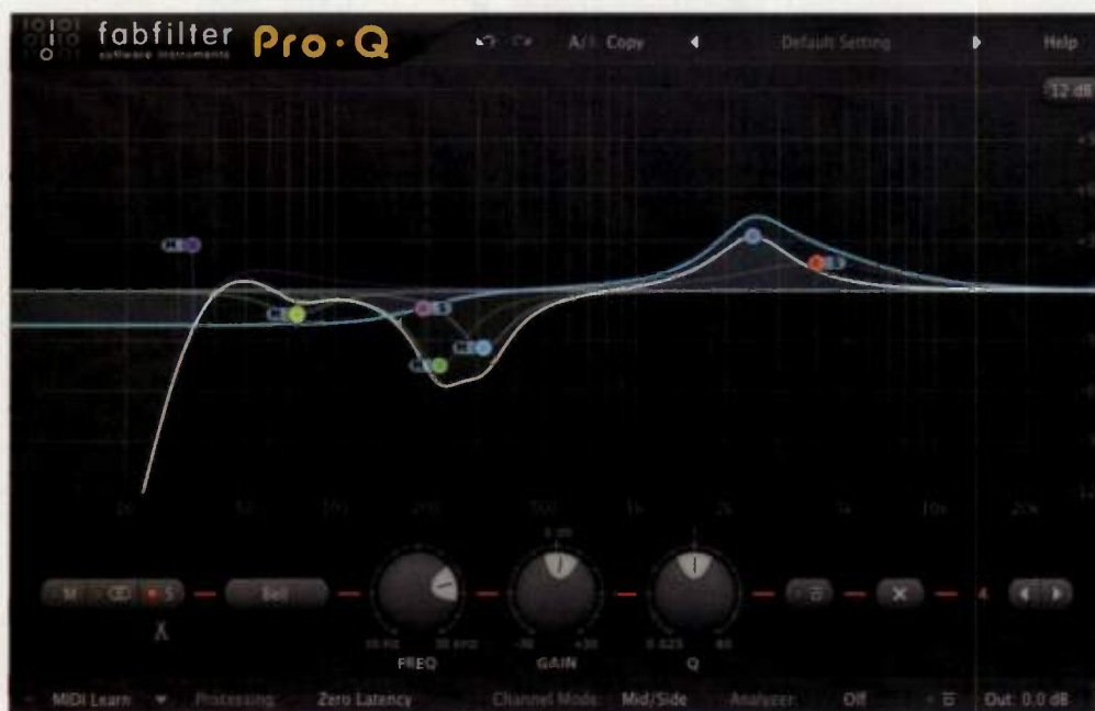
Fig. 5. Very intricate and deep mid-side equalization is applied to an extremely muddy and boomy mix, using FabFilter Pro-Q to restore clarity and add punch.
