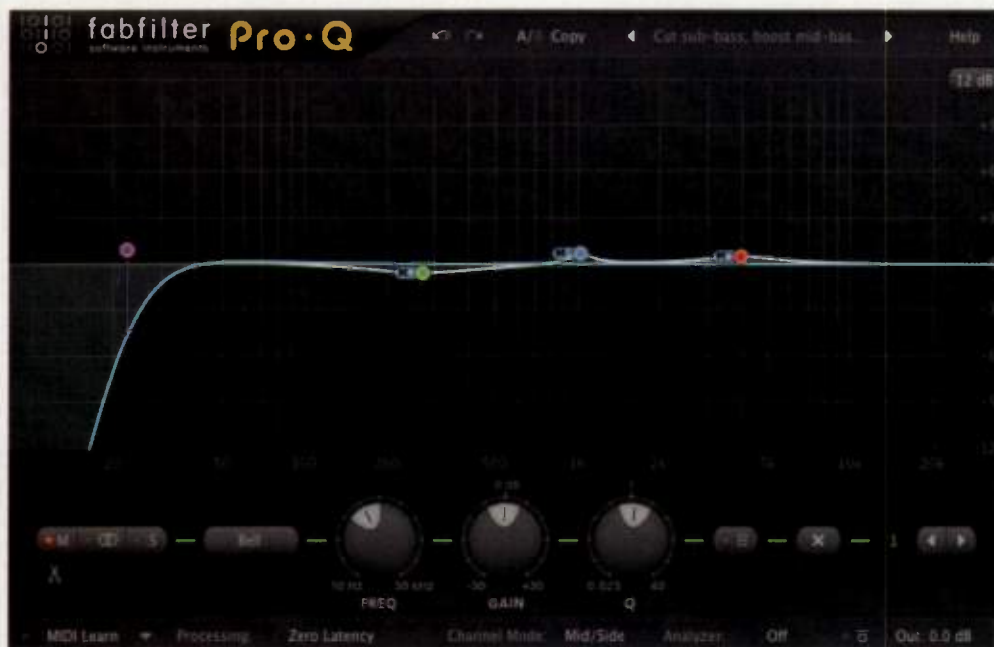
Fig. 4. Very mild bell-curve EQ is applied to only the mid channel of a well-mixed electronica track, using FabFilter Pro-Q. (The title of the custom preset no longer reflects the control settings, as the preset was edited substantially.)
