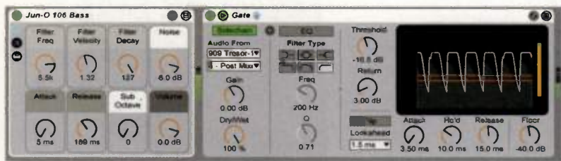
Fig. 4. Live's stock Gate on a looping bass patch, set to open on the sidechain input from the kick drum.
