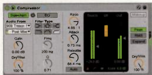
Fig. 2. Live’s stock Compressor on a bass group track with the sidechain input set to the kick drum. The Ratio is noticeable but not extreme, and the Attack is slightly open to allow some bass transients.
