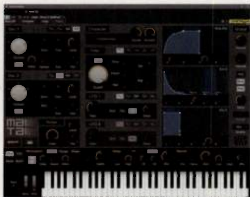
Fig. 2. The new Mai Tai synth includes the Character section, which lets you introduce unusual timbral qualities. The Envelope section allows you to adjust the curves of the envelopes manually.
