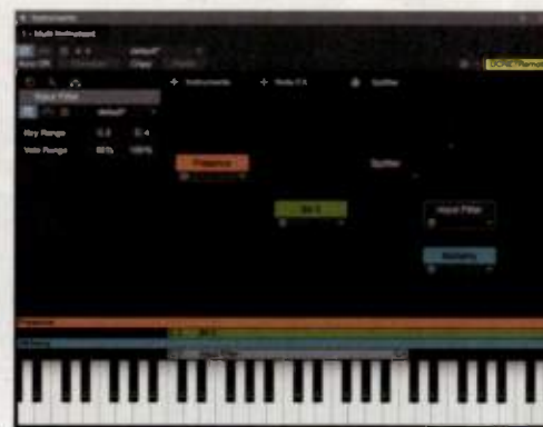
Fig. 4. Anatomy of a Multi: I have combined three Instruments by dragging a Splitter to isolate the Camel Audio Alchemy patch and a Note FX Input Filter to limit its Velocity to the upper 15 percent range.
