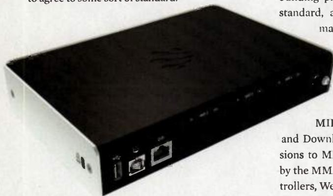
Fig 1. Because it furnishes MIDI connections via Spin DIN, USB, and Ethernet, iConnectivity's iConnectMIDI4+ is well-equipped for advances in MIDI hardware.
