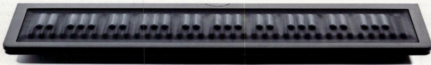
Fig. 1. The Roli Seaboard Grand is a keyboard-style controller capable of providing greater expressivity than traditional MIDI keyboards.
