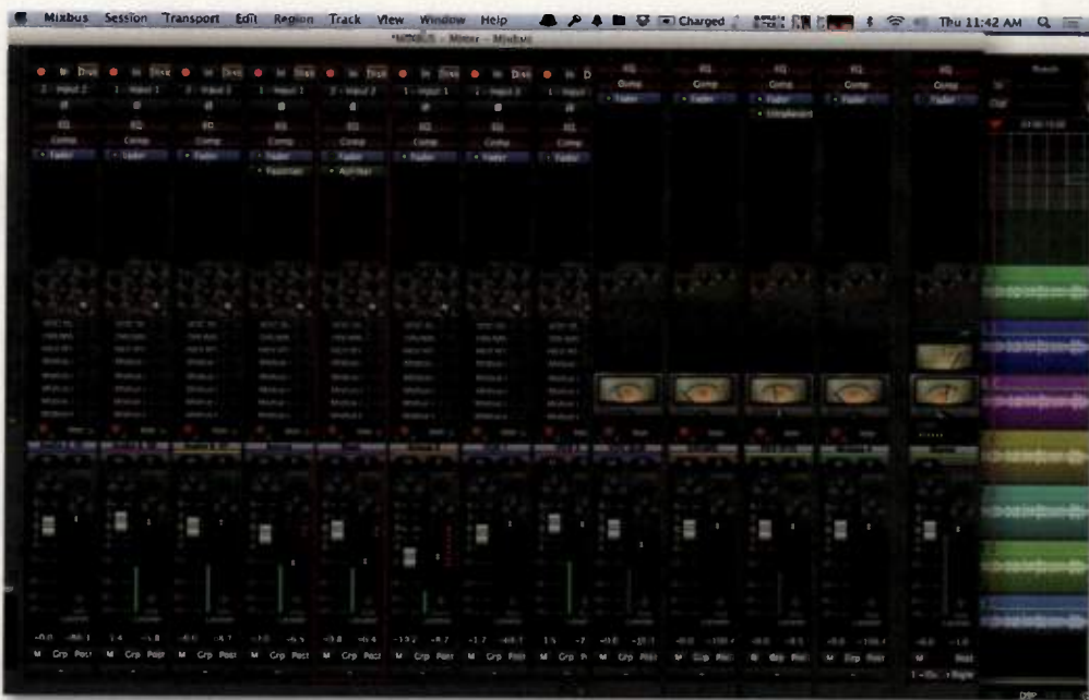
Fig. 1. The Mixer window in Mixbus 3: Tracks are on the left, while buses are located on the right.
