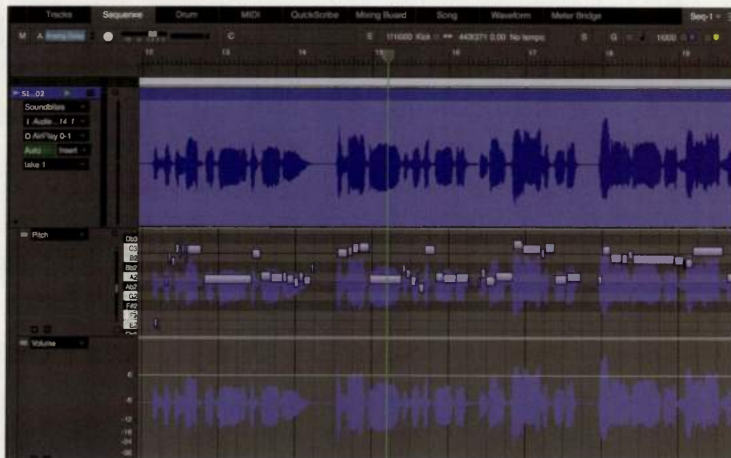
Fig. 3. Automation Lanes, such as these two for Pitch and Volume, can be opened underneath a track's main lane.
