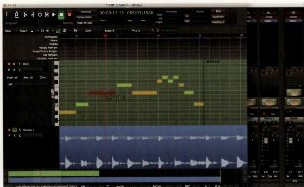
Fig. 2. Expanding a MIDI track vertically reveals a piano-roll-style editor.
