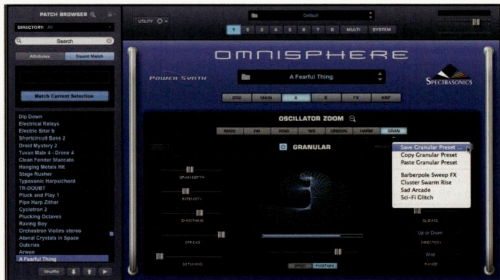
Fig. 2. Omnisphere 2 lets you use your own recordings as source material and save and recall granular-synthesis presets.
