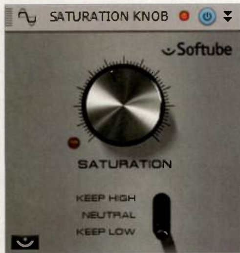
Fig. 7. Softube's free Saturation Knob modeled-distortion effect features a three-way switch, labeled Saturation Type, that lets you apply distortion to mostly the lows or highs, or to the entire frequency spectrum.
