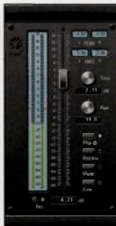
Fig. 8. Sonalksis FreeG provides a long-throw fader, peak and RMS meters, pan and trim controls, and switches to invert polarity, mute signal, and bypass.
