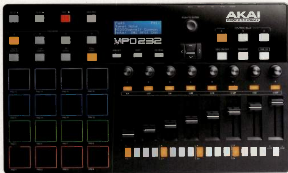
Fig. 1. The MPD232's generous control array looks even better when you factor in the four pad banks and three control banks for the knobs, faders, and buttons.
