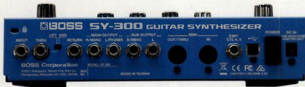
Fig. 2. In addition to standard guitar input, the SY-300 provides an effects loop, Main and Sub stereo outputs, MIDI In and Out/Thru, and a USB port. However, the unit does not do pitch-to-MIDI conversion.
