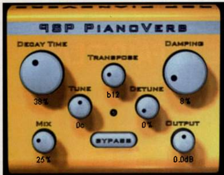
Fig. 5. PSP's PianoVerb, a stripped-down version of PianoVerb2, produces unique reverberation using twelve string operators tuned to different notes.
