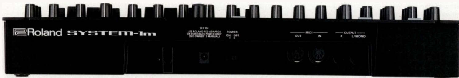
Fig. 2. The top of the System-1m provides MIDI I/O, stereo 1/4" output, and the DC input and power switch. If you rack the module and lose access to these connections, no problem: You'll find MIDI I/O on the back and audio outputs on the front, and you can power the unit from your Eurorack case or from a powerstrip.
