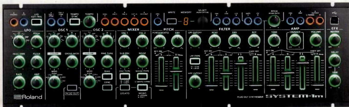
Fig. 1. Although the front resembles the System-1 keyboard, the System-1m provides a row of 3.5mm jacks that includes CV, envelope, and gate connections for use with standard modular synth gear.
