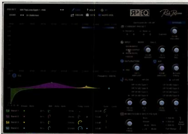
Fig. 2. RP-EQ's mono/stereo split filter lets you apply processing to lower and higher frequencies separately, and the Air section offers a wide additional band with a center frequency between 30 and 40 kHz.
