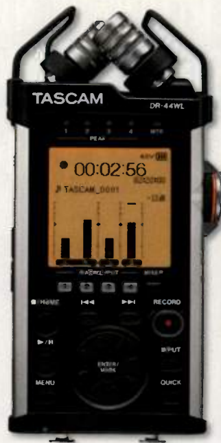
Fig. 1. The Tascam DR-44WL is a 4-track digital recorder that includes a pair of external mic/line inputs.
