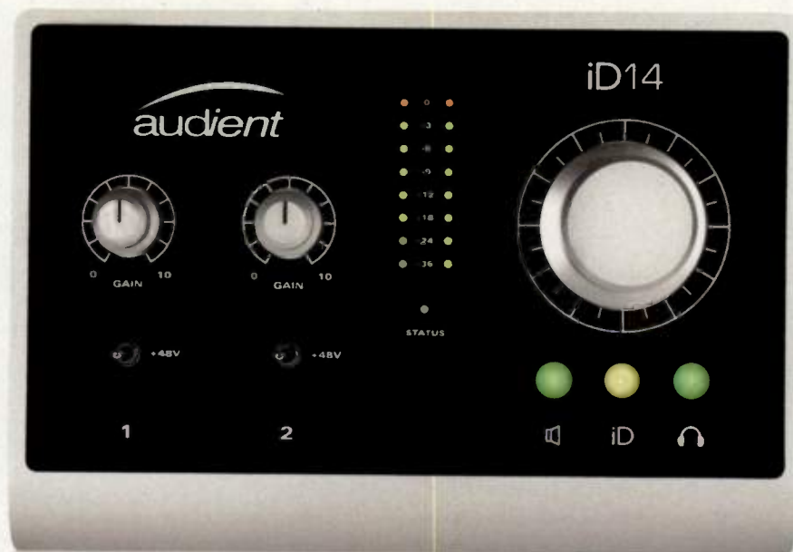
Fig. 1. All the iD14's physical controls are available from the top panel.
