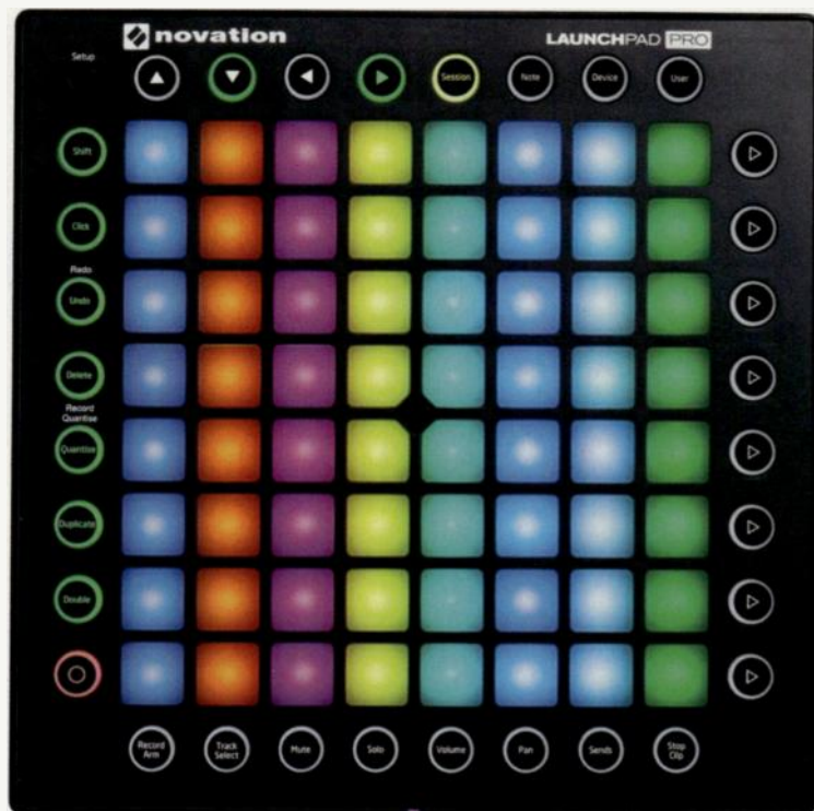
Fig. 2. The Launchpad Pro's pads now have velocity sensitivity and Aftertouch. New function buttons make recording and mixing in Ableton Live 9 much more mouse-free.
