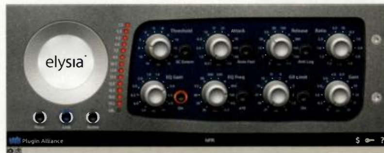
Fig. 3. The elysia mpresor's negative ratios can be used to create extreme ducked-reverb effects.
