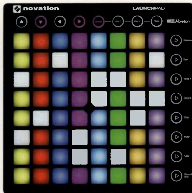
Fig. 1. The Launchpad MkII, like the Launchpad Pro, adds full RGB backlit pads to match the color of your Session View clips exactly in Ableton Live 9.
