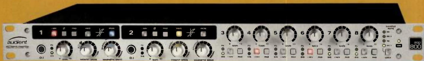
Fig. A. The ASP800 connects to the iD14's optical input, adding eight input channels (two with DI and coloration features).
