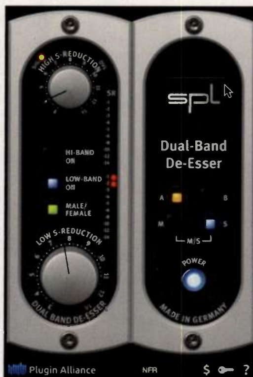
Fig. 2. For more demanding de-essing applications, the Dual-Band De-Esser allows processing in two frequency bands at once.
