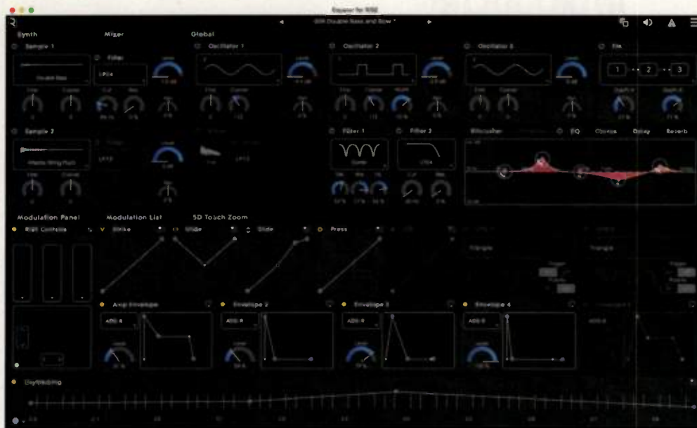
Fig. 2. Roli's Equator software for the Seaboard Rise provides mapping for all five performance dimensions. It includes two sample playback modules, three wavetable oscillators, FM synthesis capabilities, and effects.
