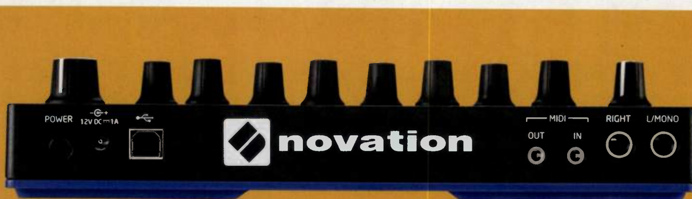
Fig. 2. Circuit comes with a wall adapter, as well as six AA batteries. The USB port is currently for sending MIDI to a computer only. Included MIDI breakout cables give you MIDI DIN I/O connections to external gear.
