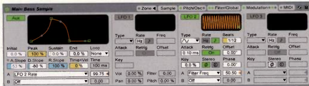
Fig. 7. Perhaps the heart of the bassline, the Aux envelope mimics the Pitch Envelope and modulates the LFO 2, which modulates the Filter Frequency.
