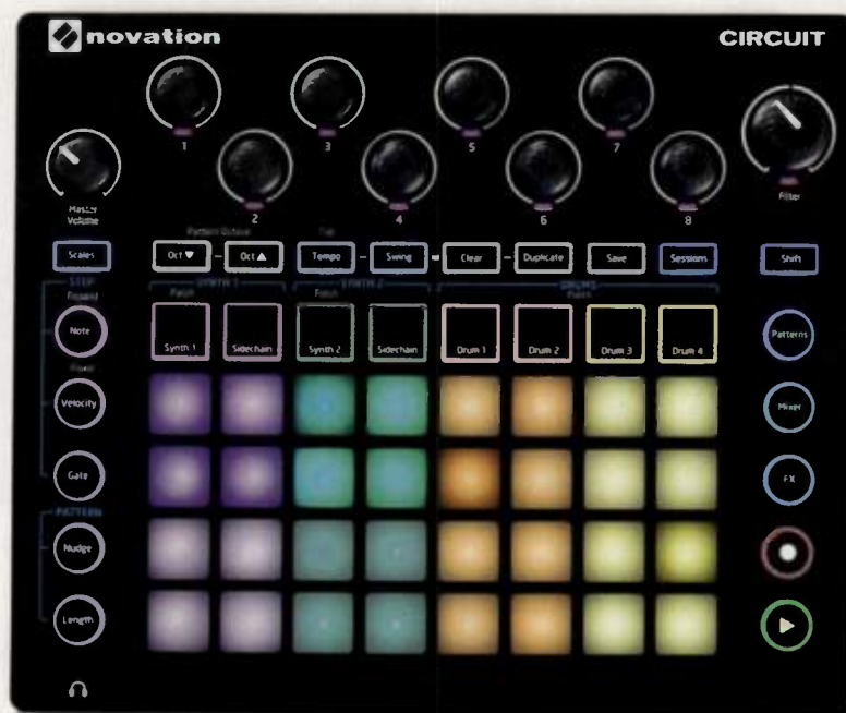
Fig. 1. Circuit's fully RGB velocity-sensitive pads use well thought out color coding, dimming, and blinking to effectively supply the compact surface with copious amounts of control interfaces.
