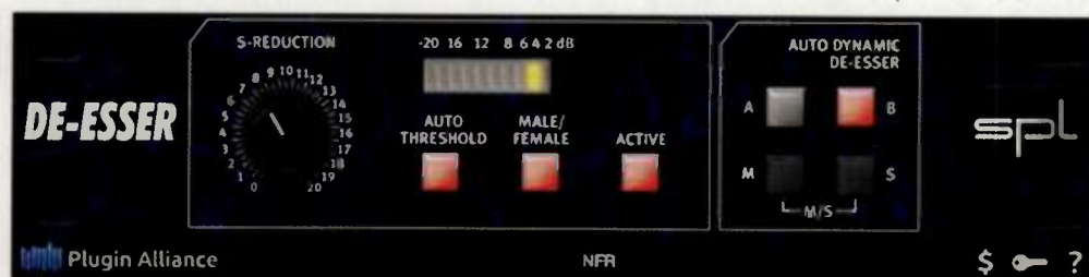
Fig. 1. The SPL De-Esser uses phase-cancellation to tame sibilance in a single frequency band.
