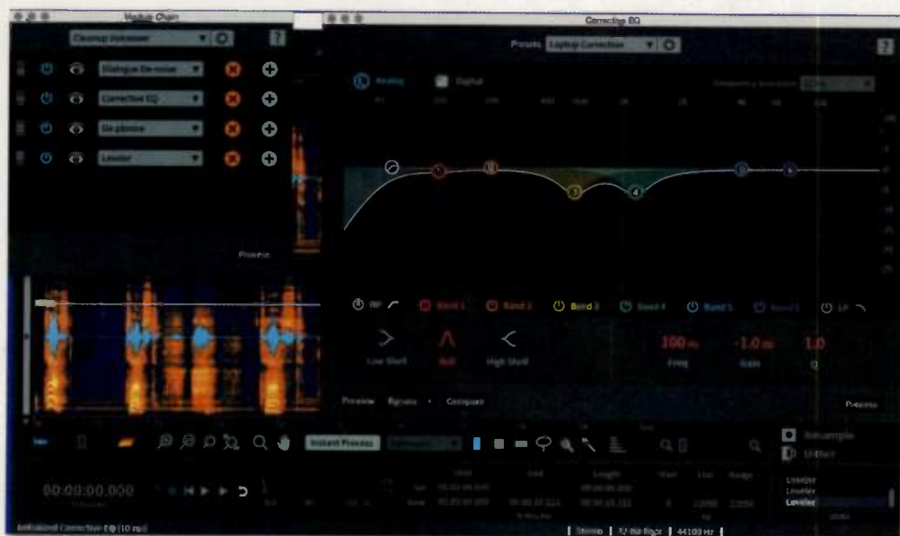
Fig. 1. Two of the modules that have been added to both versions of RX 5: Module Chain (left) and Corrective EQ.
