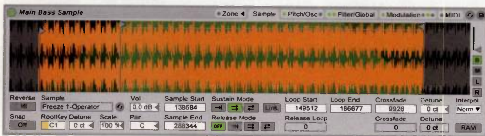
Fig. 4. The Main Bass sample has been cropped and looped with crossfading in Live 9's Sampler.
