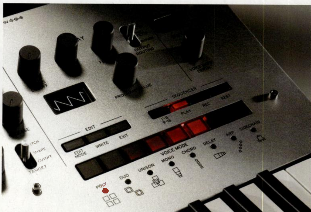
Fig. 2. A close-up of the minilogue's Voice Mode buttons, sequencer, and LCD showing an Init waveform that's ready for you to edit into a new patch.
