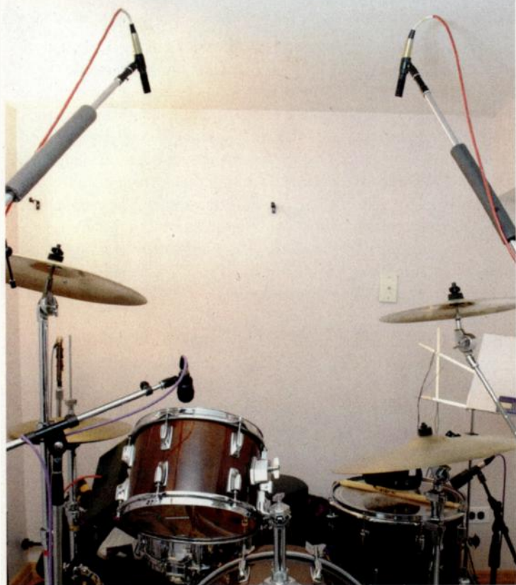
Fig. 4. Try miking a kit with a spaced microphone pair, placing mics about six feet high, four to five feet apart, and pointing straight down at the floor.
