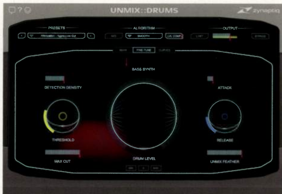
Fig. 1. Zynaptiq Unmix::Drums can transparently boost or attenuate drums in a prerecorded mix. The GUI's Fine-Tune view is shown here.
