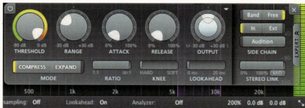
Fig. 2: Detail of compressor controls: Use a hard knee and high ratio and threshold settings.
