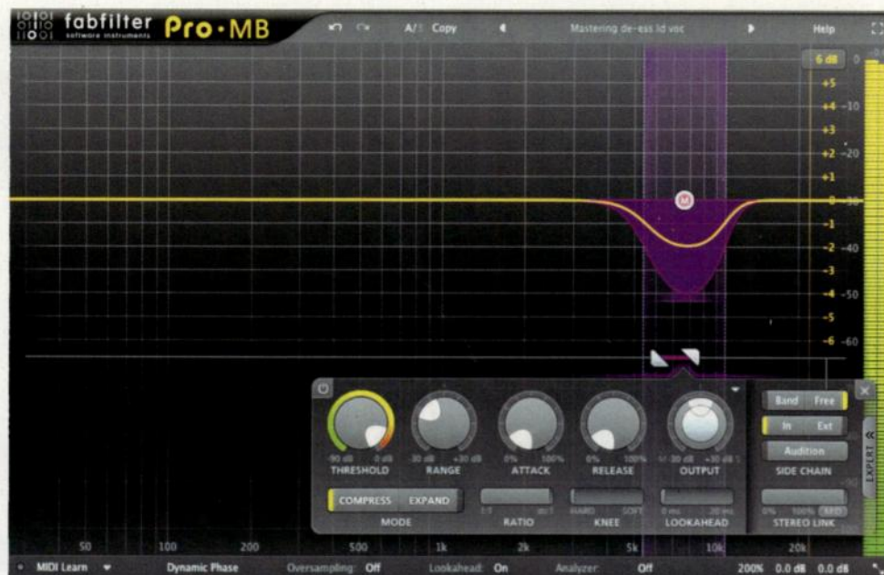
Fig. 1: To de-ess vocals in a full mix—and prevent instruments from triggering compression—set the band-pass filter in FabFilter Pro-MB's sidechain to a narrower bandwidth than the filter in the mid channel's audio path.
