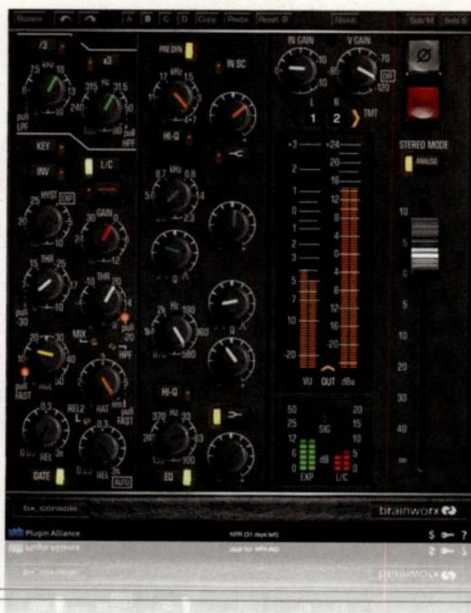
Brainworx bx_console emulates the rare Neve VXS mixing board. It includes 4-band EQ, a limiter/compressor, and a gate/expander.
