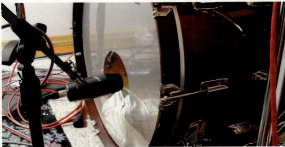
Fig. 1. To record kick, start with a single dynamic mic placed so that most of the body is outside the drum, and the grille is just inside the resonant head's hole.
