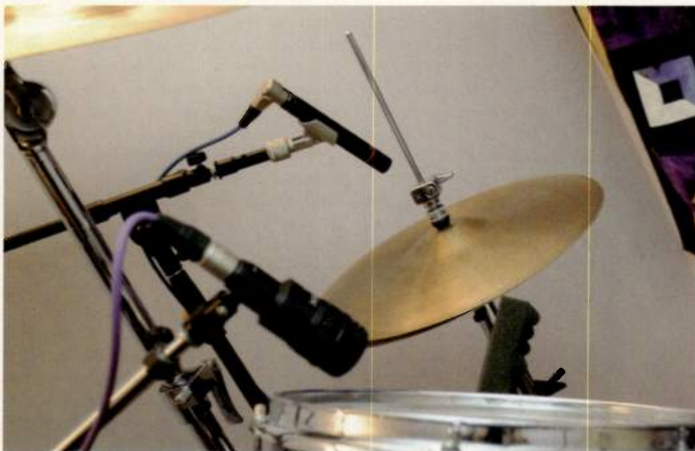
Fig. 5. Hi-hat mic placement. Here, the mic is pointing away from the kit to reduce leakage, but captures plenty of “chick” from the cymbals.
