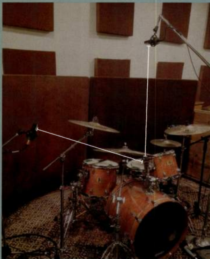
Glyn Johns' Mic technique. Note distance from each mic to snare must be identical.
