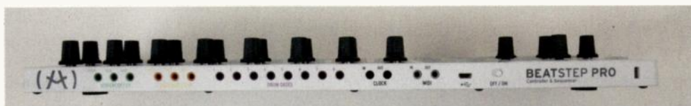
Fig. 2. Plenty of CV/gate, MIDI and Clock sync connections mean the BeatStep Pro can wrangle together just about any music gear into a cohesive performance troupe.
