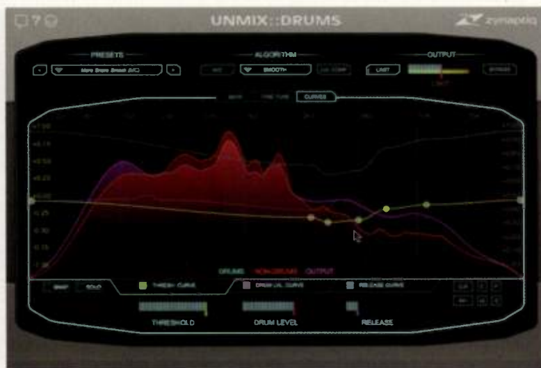
Fig. 2. The Curves view allows breakpoint editing for Threshold, Drum Level, and Release controls on an XY plot, shaping powerful frequency-dependent processing.
