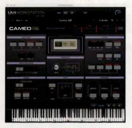
Fig. 3. Notice the knob just below the patch window in the CM synth: Use it to select any of 33 available waveforms. Furthermore, you can assign MIDI messages to sweep the table. Just below the amplitude ADSR is a slider to add or decrease phase distortion.
