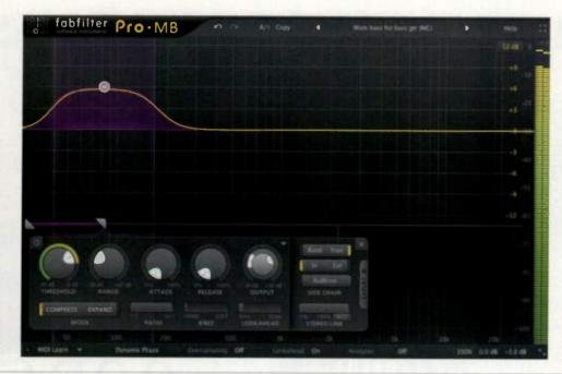
Fig. 1. When adjusting the output-gain control for a filter assigned to the mid or side channel in FabFilter Pro-MB, use the filter's pan control to reverse the gain change in the opposing channel.
