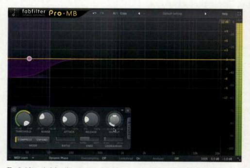
Fig. 2. A low-shelving filter's pan control (see mouse pointer) is used in Pro-MB to collapse a mix's bass frequencies to mono. The filter's Range control has no effect on the bass band's panning to center and is set to -6 dB here solely to make the filter's bandwidth more apparent for illustrative purposes.
