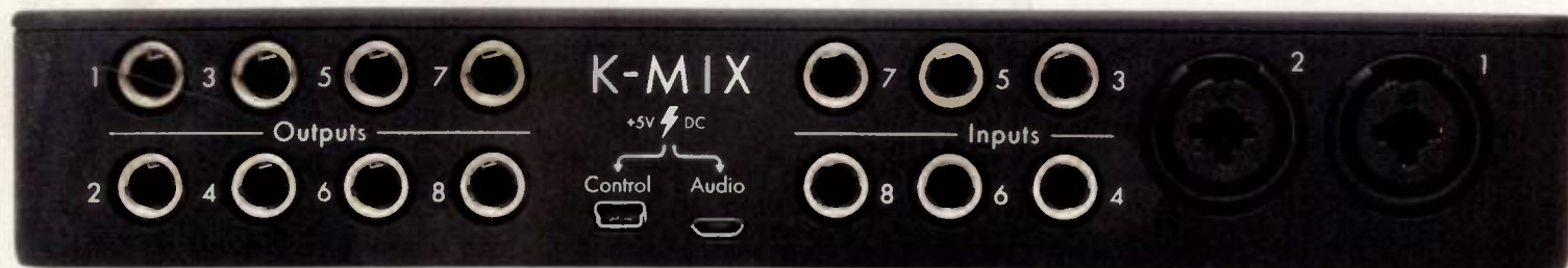
Fig. 2. K-Mix offers a generous amount of analog I/O, and the outputs can easily be configured for surround applications. Inputs 1 and 2 accept mic-, line-, and instrument-level input.
