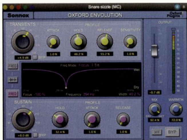
Fig. 2. Separate, adjustable filters for the transient and sustain envelopes affect both their detection and the frequencies that are processed for each. A broad notch filter for the sustain envelope is shown here.
