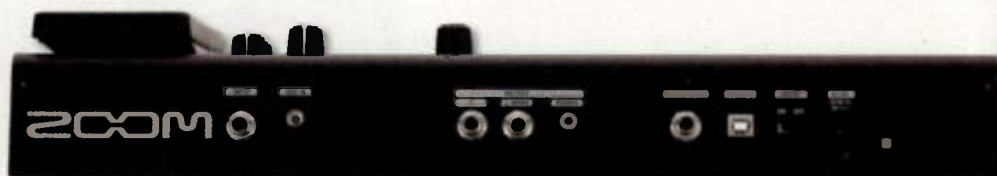
Fig. 1. The rear panel shows the G5n's I/O, which gives you what you need to use the unit, but no effects loop or MIDI ports.
