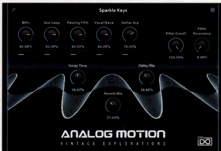
Fig. 2. In Falcon's Info view, each program displays a unique panel of controls defined by its programmer. Because a single macro can simultaneously control numerous parameters, you can name them anything you like.
