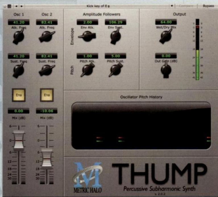
Fig. 1. Metric Halo Thump can generate multiple subharmonics that sound fantastic on drum tracks. Here, Thump's two oscillators are tuned to E notes an octave apart.
