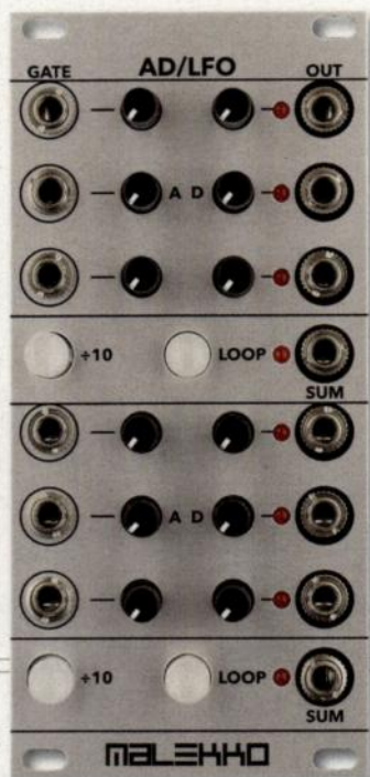
The DSP-based AD/LFO is a 6-channel envelope generator that can be configured into two sets of three LFOs. A combined signal of each set of three CV outputs is available at the Sum output jacks.
