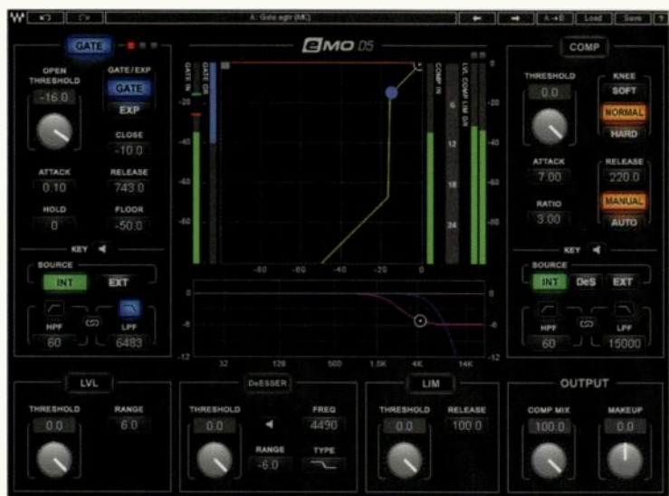
Fig. 2. You can prevent the gate in Waves' eMo D5 plug-in from chattering by setting an offset for the closing threshold with respect to the opening threshold. The Close control (in the upper-left section of the GUI) adjusts the offset in decibels.
