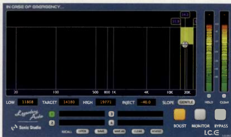
Fig. 2. I.C.E. is used to boost energy in a mix's top octave.
