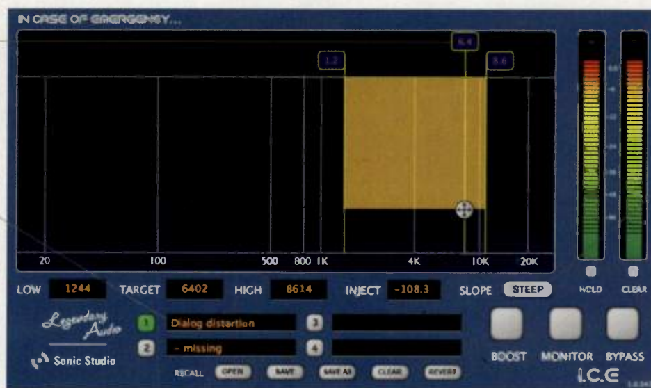
Fig. 1. I.C.E. addresses distortion occurring within an adjustable frequency band. The gold bar to the left of the meters shows the amount of processing applied in the band.
