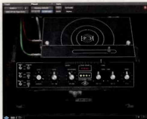
Fig. 2. The Universal Audio EP-34 Tape Echo plug-in with the Repeats control set high enough to produce self-oscillation and a delay time of 628 ms.
