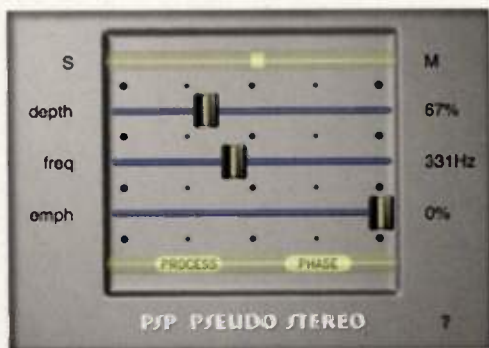
Fig. 3. PSP PseudoStereo's controls adjust the perceived width and relative amount (vs. mono input) of its stereo effect. The yellow square seen here at the top of the GUI expands horizontally and moves to the right or left as the plug-in's output becomes more correlated (right) or decorrelated (left).
