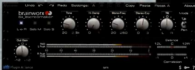
Fig. 1. Brainworx bx_stereomaker includes controls for centering bass frequencies, reducing highs in and panning the differential signal, panning the mono source, and adjusting the tone and width of its stereo effect.
