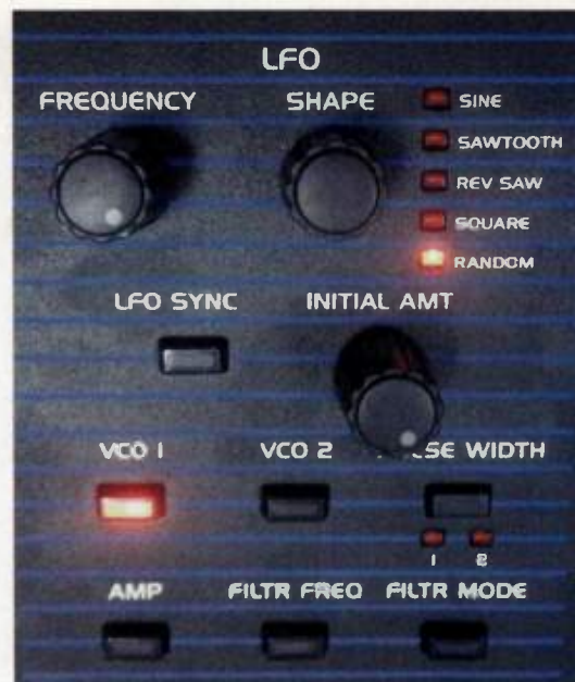
Fig. 5. Using the LFO to modulate noise
