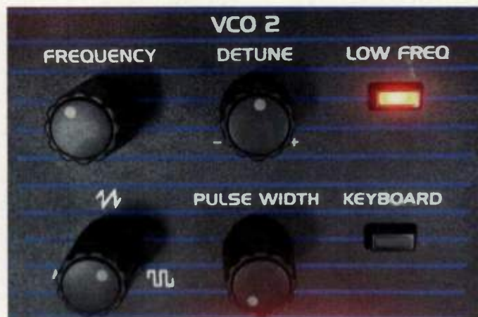
Fig. 4. Using VCO2 as a second LFO
