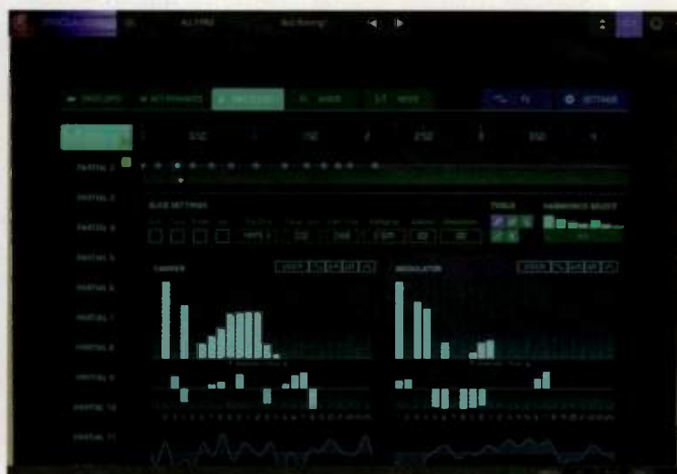
Fig. 6. Synclavier V's Screen window emulates Synclavier's Green Screen. You can deploy up to 50 time-slice frames, consisting of individual timbres shaped by a combination of Additive and FM synthesis, for each of the 12 Partials. The small circles at the top represent the sliced frames as they are positioned in the timeline.
