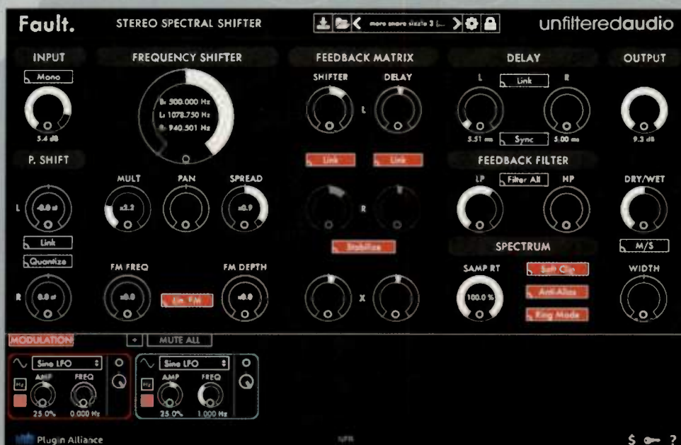
Fig. 1. Fault's dual frequency shifters and delay lines add a virtual bottom mic to a snare track for added sizzle.
