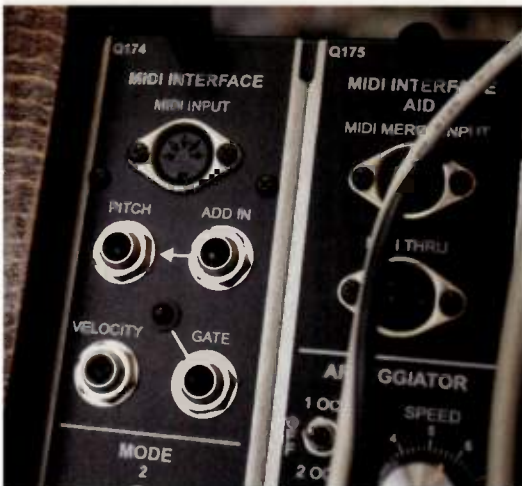
Fig. 5. A Modern MIDI interface providing a 5-volt Gate output, along with pitch and velocity
