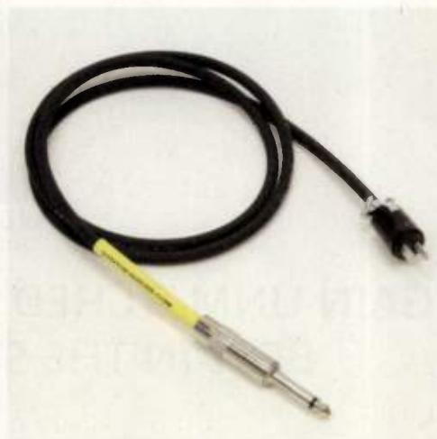
Fig. 4. A simple cable providing a passive circuit conversion from Gate (Voltage-Trigger) to Switch-Trigger
