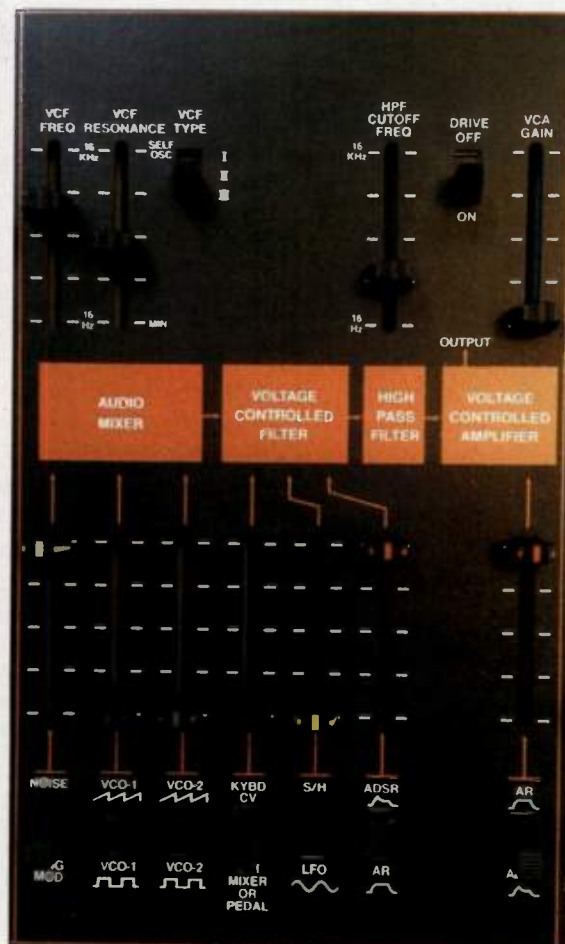
Fig. 3. The Filter module includes the mixer section (with ring mod selected and set to maximum). Note that oscillator waveshapes are selected here, instead of on the oscillator itself.
