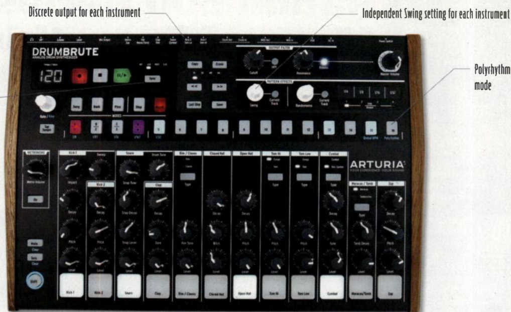
Fig. 1. DrumBrute supplies 17 full-bodied analog drum and percussion sounds across 12 channels, and includes an analog highpass/lowpass filter, 64 internal patterns, and powerful pattern effects.
