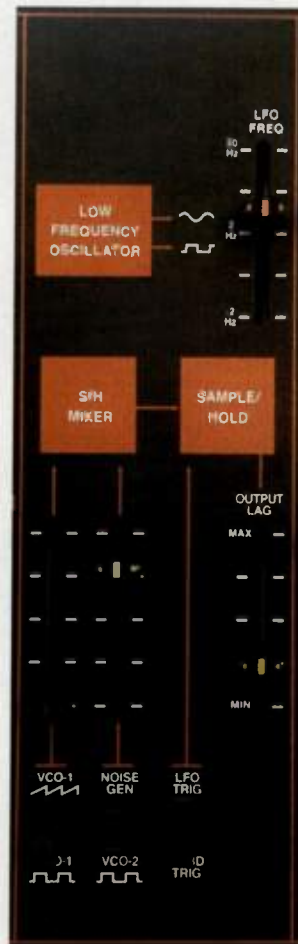
Fig. 2. The Odyssey's S/H section is capable of modular-like routing of modulation signals. Here, it's configured for classic "random" effects, with a touch of lag for that R2D2 sound.
