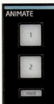
Fig. 3. Peak's LFOs include a unique parameter that controls the number of repeats up to 127. When set to off (shown here), the LFO functions traditionally.
