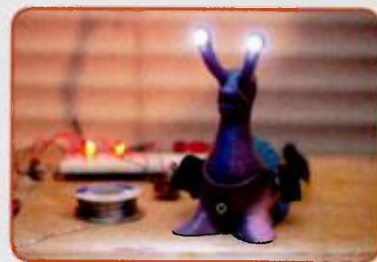
Fig. 3. I drilled out the eye stalks in this giant slug monster and inserted LEDs that pulse in sync with the two oscillators inside. The left knob is wired backwards so turning it toward the head raises the pitch.
