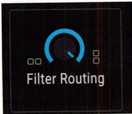
Fig. 12. With a little pre-planning, you can route each engine to its own filter for layered effects, like those on Roland's D-50
