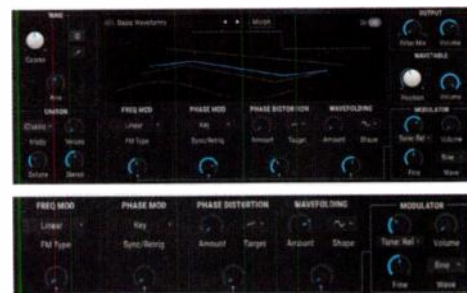
Fig. 5. Wavetable includes four vintage synthesis tools: FM, Phase Modulation, Phase Distortion, and Wavefolding.
