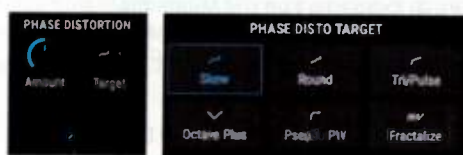
Fig. 8. Pioneered by Casio, Phase Distortion can transform a sine wave into a harmonically rich waveform. Pigments includes six waveshape targets for this process.
