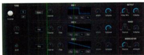
Fig. 1. Based on the Minimog architecture, the Analog engine includes three oscillators, sync, and blendable modulation from Osc 3 or Noise
