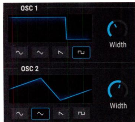
Fig. 4. The Width parameter applies to both pulse-width and triangle-saw transformations
