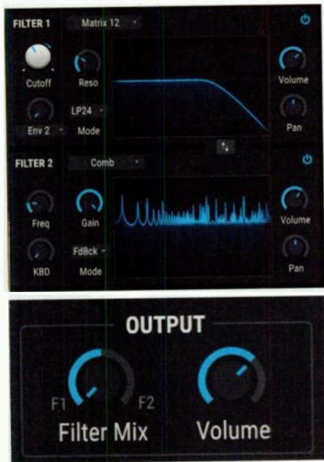
Fig. 10. Pigments' dual filters can be arranged in series, parallel, or a blend of the two routings
