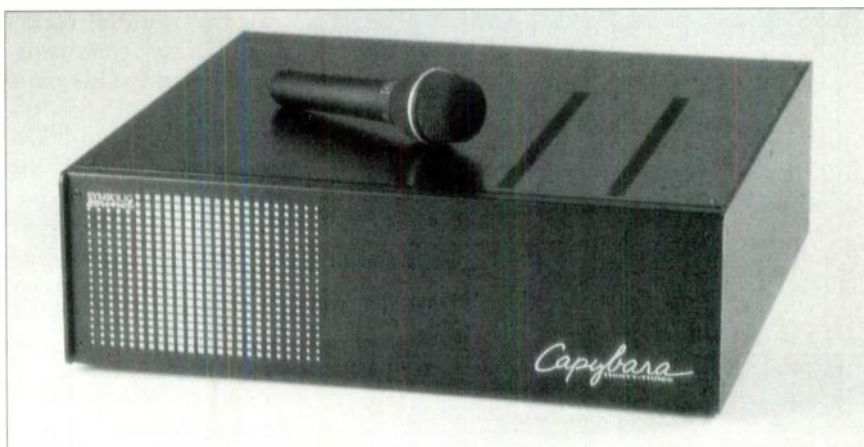
The Capybara contains the Kyma System's audio I/O and MIDI ports and accepts up to eight DSP expansion cards.
