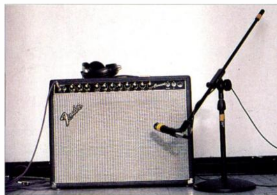
To capture a classic guitar roar, a Shure SM57 was positioned six inches off-axis from the speaker cone of a Fender Concert combo amp.
