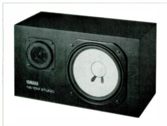
When using 2-way, near-field reference monitors, the best stereo imaging is maintained when the speaker is placed on its side. The woofers should face inside and the tweeters outside.
