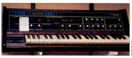
Count your blessings! This EML Syn-Key, one of the first programmable synths, used plastic program cards like the one on the left. Users punched holes in the cards to represent data in 3-bit binary numbers.
