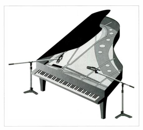
FIG. 2: To capture a stereo spread when miking a piano, angle a dynamic mic toward the bass strings and a condenser toward the treble strings.
