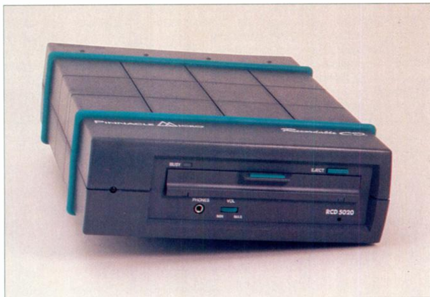
The Pinnacle RCD 5020 supports disc-at-once recording, track offsets, and intertrack index points. However, discs burned with the 5020 occasionally didn't play back properly on other machines.
