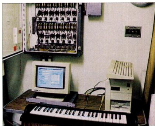
FIG. 1: The bell tower's old system (top photo) was centered around a rotating drum with prongs that physically triggered the bells. The new system (bottom photo) sports a slick MIDI design programmed in Visual Basic, sequenced in Cubase Lite , and triggered via the Leprecon.
